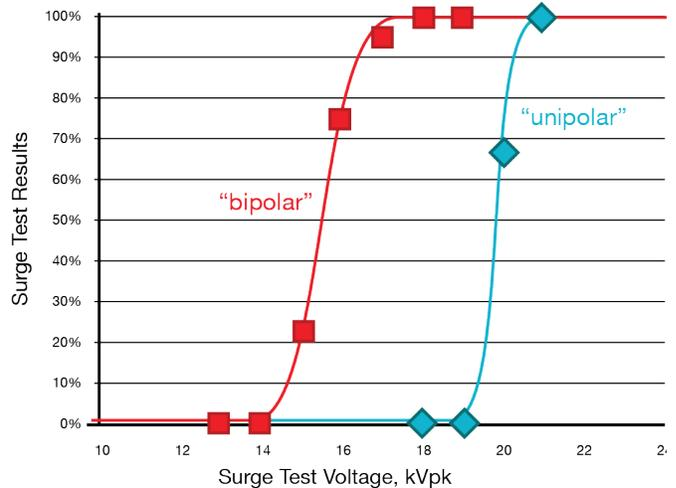
**Figure 7.** Surge breakpoint statistical assessment, by both “unipolar” and “bipolar” surge test methods .
