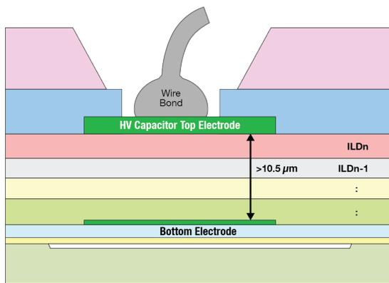
**Figure 1.** HV capacitor.
