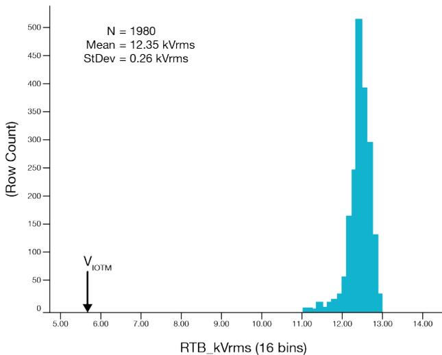
Figure 4. RTB voltage distribution, with 1 kVrms/sec ramp rate.
