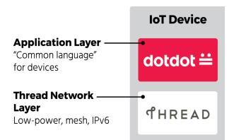
*Figure 2:* Thread and Dotdot application layer. Image source: Zigbee Alliance (www.zigbee.org)
