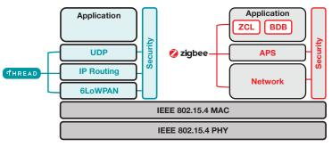
Figure 1. Zigbee and Thread protocol layering.
