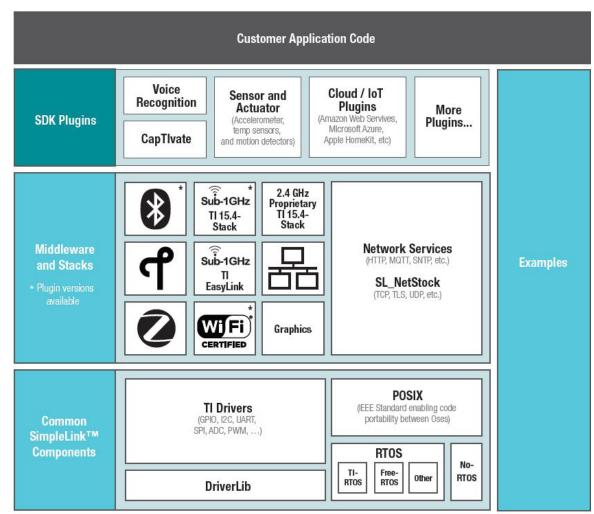
Figure 3. SimpleLink SDK diagram.
