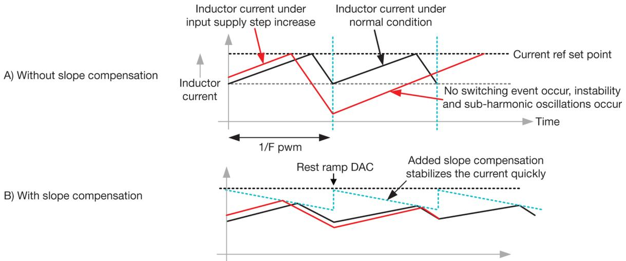
**Figure 4.** Peak Current-mode Control Implementation with Slope Compensation.
