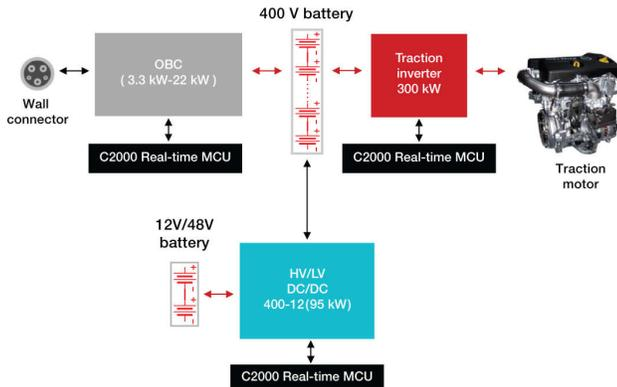
**Figure 1.** EV Powertrain System Block Diagram.
