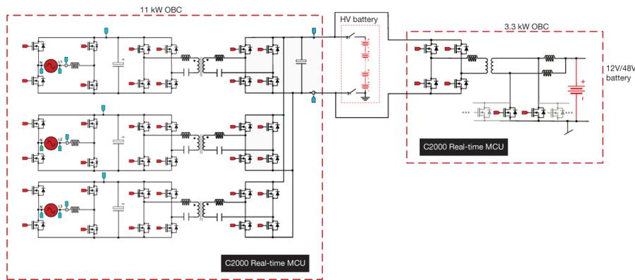
**Figure 5.** 11-kW OBC with 3.6-kW Stacked Chargers and a High-voltage to Low-voltage DC/DC Converter.
