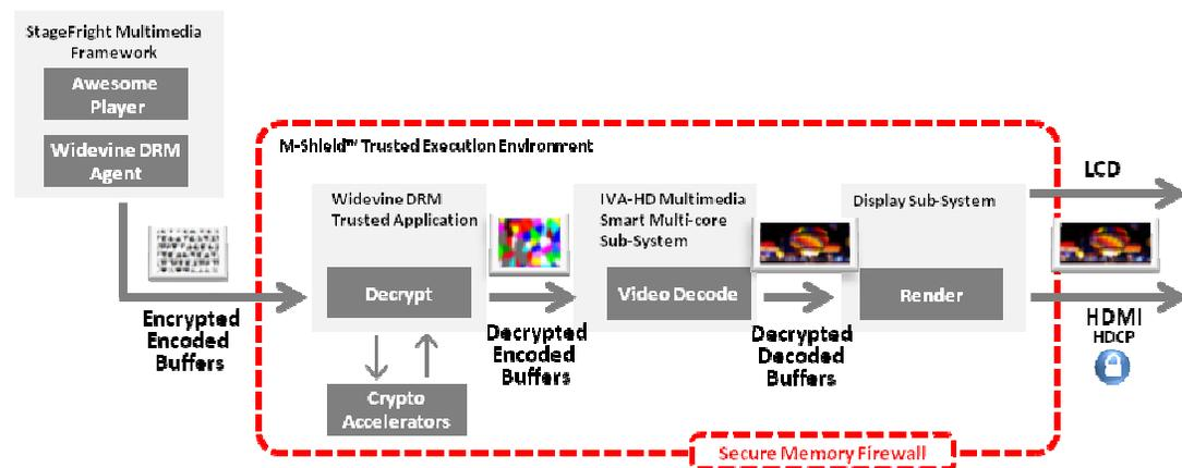
**Figure 6** - OMAP 4 Platform HD 1080p Secure Video Playback
