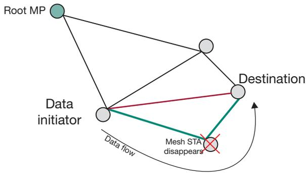
Figure 7: Mesh network where mesh device disappears
