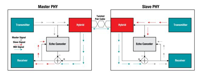
Figure 4. Echo cancellation and hybrid block diagram [11].
