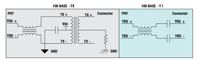
Figure 5. 100BASE-TX vs. 100BASE-T1 DC isolation.
