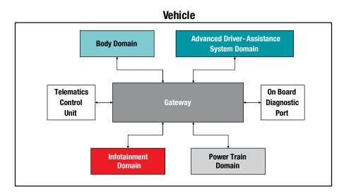
Figure 1. Gateway block diagram.
