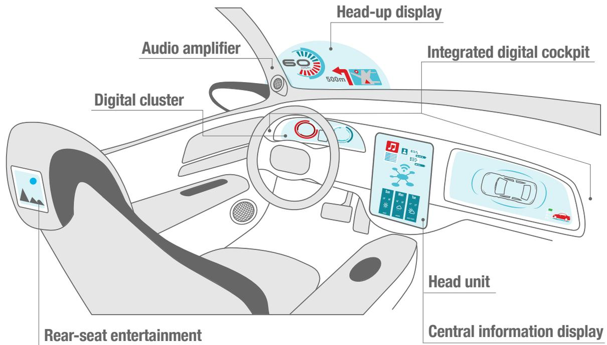
**Figure 1.** Components of an infotainment system.
