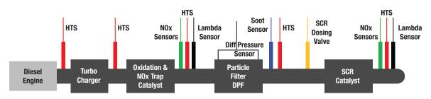
Figure 4. Types of sensors in an automotive exhaust system.
