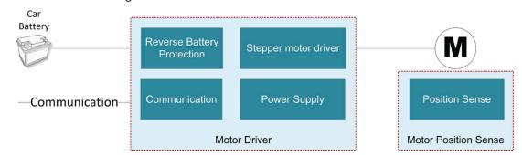
Figure 6. Block Diagram of a Stepper Motor Driver.
