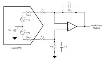
Figure 2. Audio DAC Output Circuit
