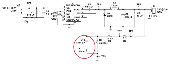
Figure 3. Application Circuit 1 Using Aluminum Output Capacitor
