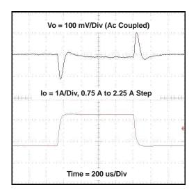
Figure 10. Measured Load Transient Response for Application Circuit 2, Vin = 12 V
