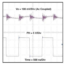
Figure 9. Measured Output Ripple for Application Circuit 2, Vin = 12 V and Vo = 5 V/3 A
