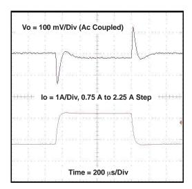
Figure 6. Measured Load Transient Response for Application Circuit 1, Vin = 12 V
