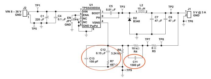
Figure 7. Application Circuit 2 Using Ceramic Output Capacitors
