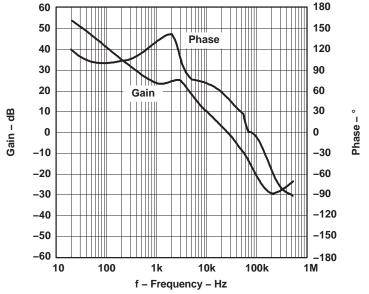
Figure 2. Measured Loop Response for TPS5430EVM-136, Vin=10.8 V
