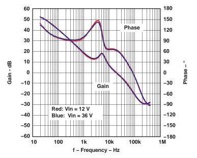
Figure 8. Measured Loop Responses for Application Circuit 2, lo = 3 A
