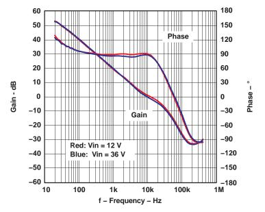
Figure 4. Measured Loop Responses for Application Circuit 1, lo = 3 A
