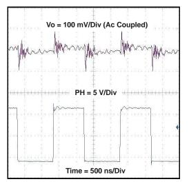
Figure 5. Measured Output Ripple for Application Circuit 1, Vin = 12 V and Vo = 5 V/3 A
