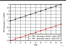
Figure 1. RH Accuracy at Time Zero Plus the Long Term Drift Over Time
