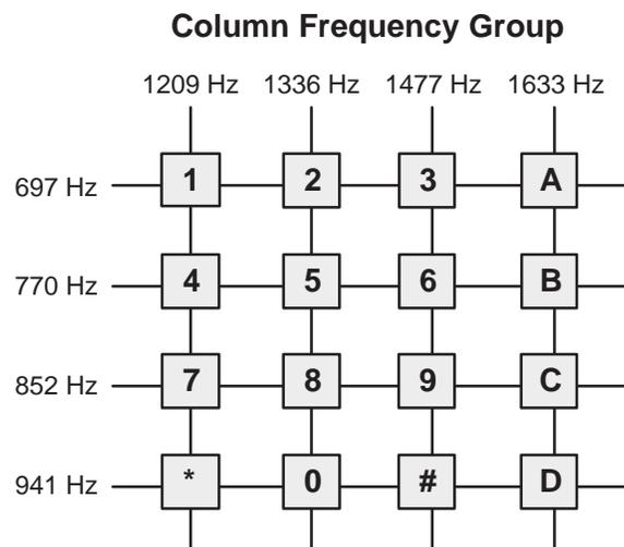
**Figure 1. Touch-Tone Telephone Keypad: A Row and a Column Tone is Associated With Each Digit**
