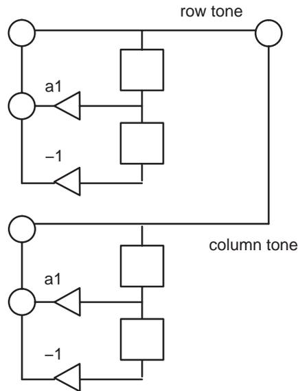
Figure 2. Two Second-Order Digital Sinusoidal Oscillators
