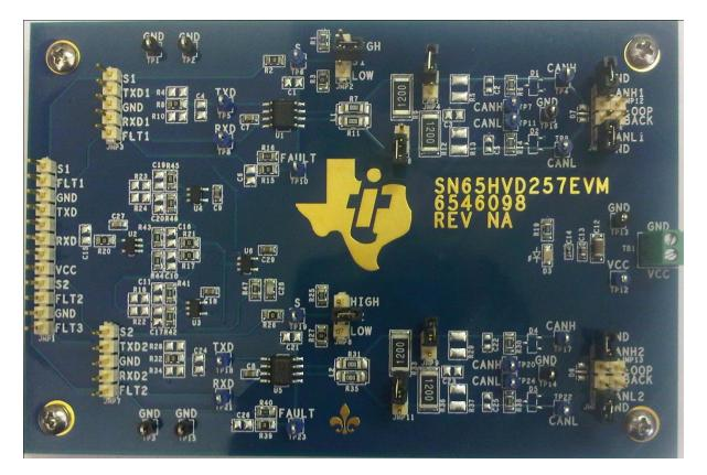
FIGURE 1. Top side of SN65HVD257 CAN EVM
