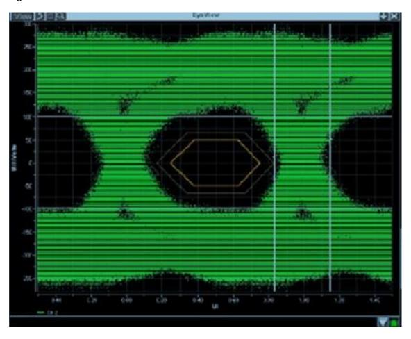
• Figure 1. Eye diagram with PCLK = 43MHz, PRE = OFF, 1m cable
