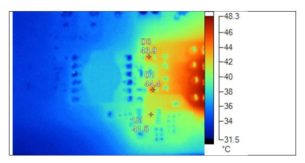
Load resistors at output 1 and 3 (right handed) are radiating to the power stage; The rectifiers and the controller are below 50c at 23c ambient temperature. The losses at output 2 and output 4 are minor, total converter losses are 163mW.
