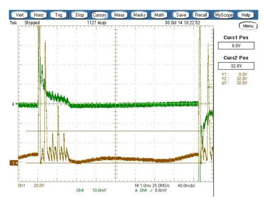
Figure 13: Current regulator drain waveform when forward phase dimming (dimmer at minimum)
