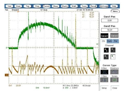
Figure 6: Current regulator drain waveform (Brown), input current (green)
