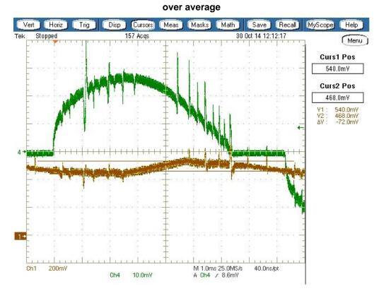
Figure 29: current ripple stack 3, 36 volt, voltage across 10 ohm resistor, approximately 14% peak to peak
