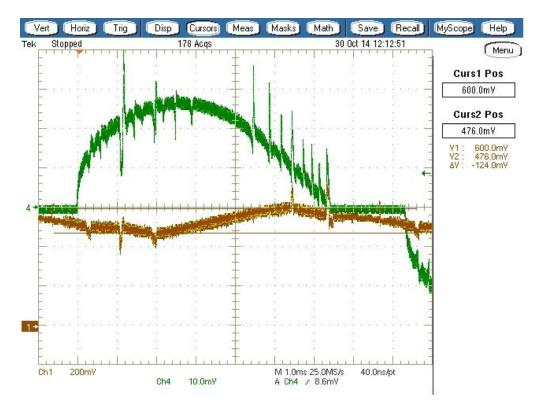
Figure 28: current ripple stack 2, 78 volt, voltage across 10 ohm resistor, approximately 23% peak to peak
