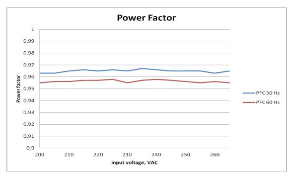
Figure 4: Power factor correction at 50 Hz and 60 Hz
