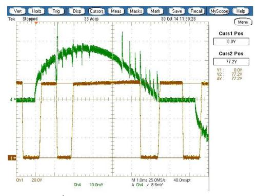
Figure 23: 2<sup>nd</sup> TPS92411 drain, 78 volt stack, x1xx in count sequence
