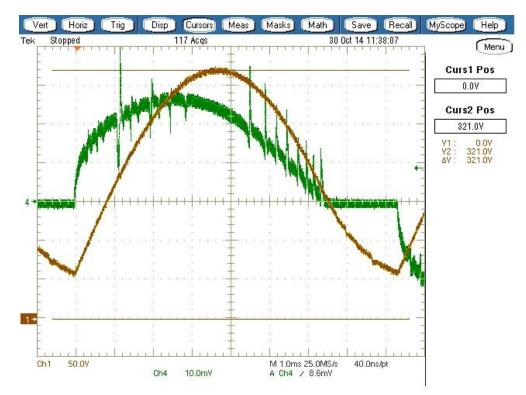
Figure 18: Rectified AC, reference for next oscilloscope plots (brown), note the line regulation circuit prevents the current regulator from sinking current when the rectified AC voltage is low
