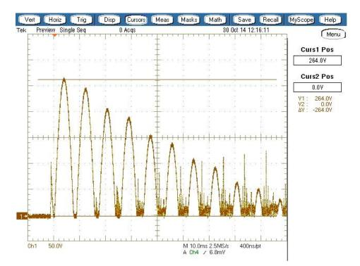
Figure 9: Current regulator drain voltage during power on, energy storage capacitors charging
