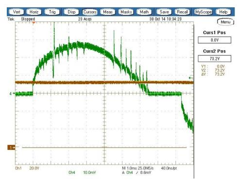
Figure 17: Input averaging voltage used for line regulation, D28 (brown)
