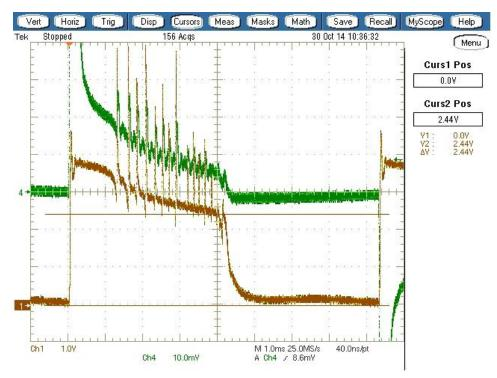
Figure 16: Current sense voltage while forward phase dimming, R15 (brown)
