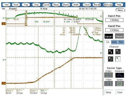
Figure 21: Drain of cascode MOSFET, open slew, 1.9V/uS
