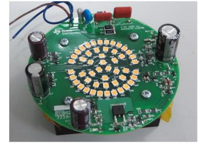
5.6 TPS92411 test hardware, designed mounting to heatsink though printed circuit board, 0.031" thick.
