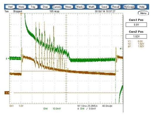
Figure 15: Current reference with DC offset, R29 (brown), shows DC offset held up by C6
