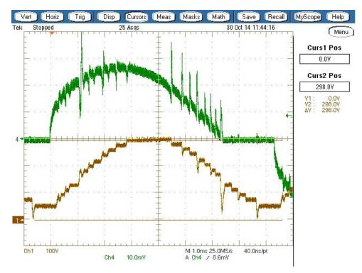
Figure 26: Series load voltage, sum of the LED stacks as the input voltage rises and falls
