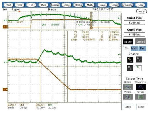
Figure 22: Drain of cascode MOSFET, close slew, -2.9V/uS
