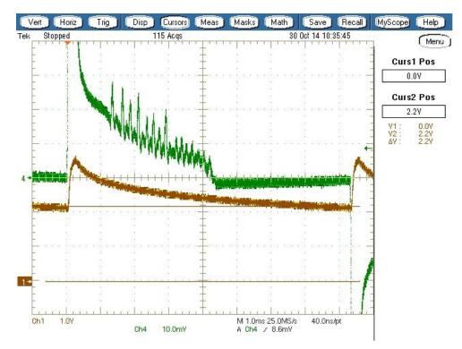
Figure 14: Voltage on DC offset circuit, C6, holding command up when forward phase dimming (brown)
