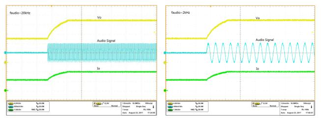
Figure 4.1 Output Voltage Transition at faudio=20kHz
