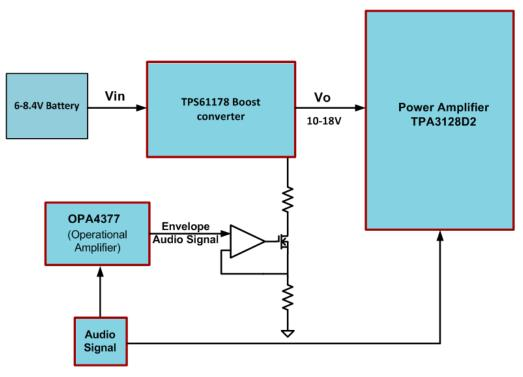
Figure 1. Block Diagram of the PMP15036
