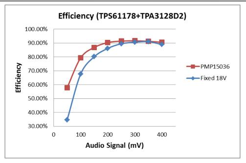
Figure 6 Efficiency Comparison Result (Vin=7.2V, Ro=4 ohm)
