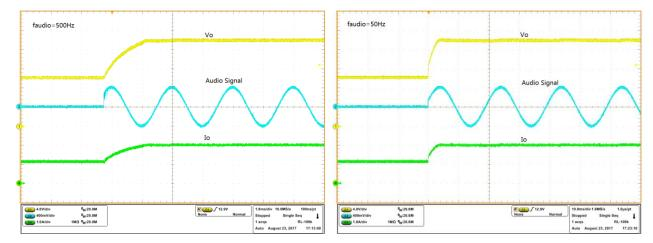
Figure 4.3 Output Voltage Transition at f<sub>audio</sub>=500Hz Figure 4.4 Output Voltage Transition at f<sub>audio</sub>=50Hz
