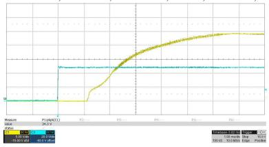
0A load, 1msec/div; CH1: Vout, 5V/div; CH2: Vin, 20V/div:
