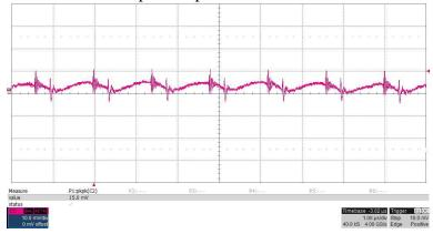
Input Ripple at C4, 10mV/div, 1usec/div Measured 14.0mVpeak to peak:
