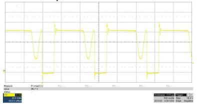
D1 Anode to GND, 57V input, 700mA load, 50V/div, 500nsec/div, 750MHz bandwidth Measured 153Vpeak:
