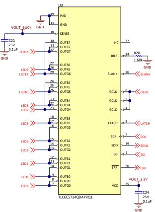
Figure 10. TLC6C5724-Q1 Linear LED Driver Schematic
