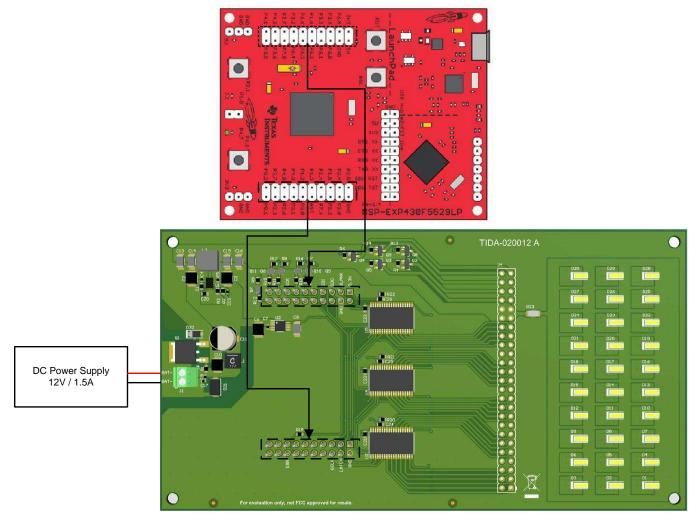
The MSP430 LaunchPad can be connected to the PCB using the headers J2 and J3. Connect a DC power supply to the input terminal J1.
