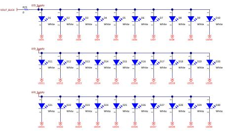
Figure 12. Schematic of 30 LEDs
