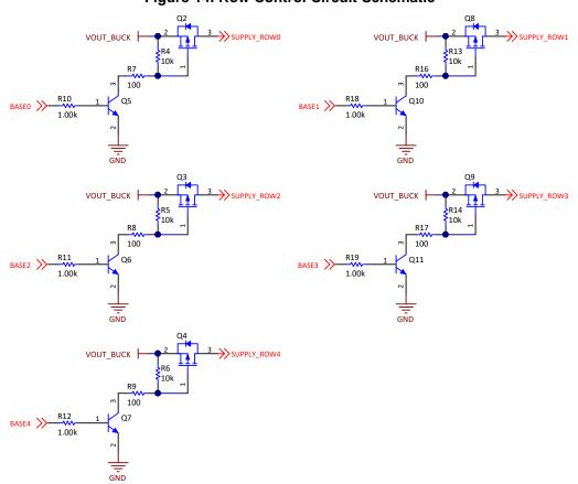
Figure 14. Row Control Circuit Schematic
