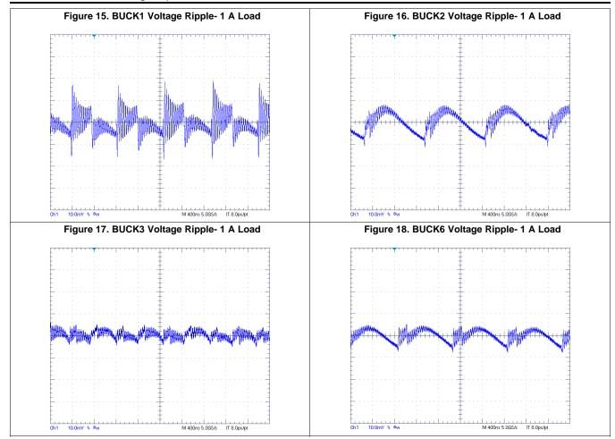
Hardware, Software, Testing Requirements, and Test Results
