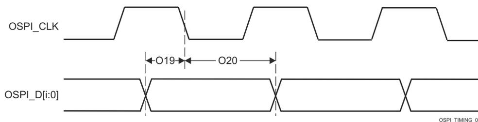
**Figure 6-105. OSPI0 Timing Requirements – Tap SDR, No Loopback**
