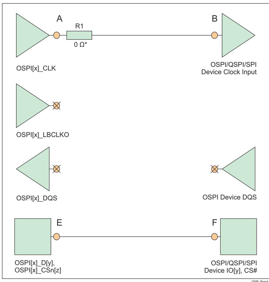
\* 0Ω resistor (R1), located as close as possible to the OSPI[x]\_CLK pin, is placeholder for fine tuning, if needed.
