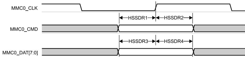
**Figure 6-69. MMC0 – High Speed SDR Mode – Receive Mode**
