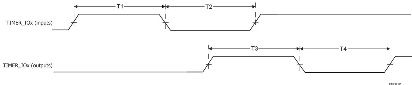
**Figure 6-109. Timer Timing Requirements and Switching Characteristics**
