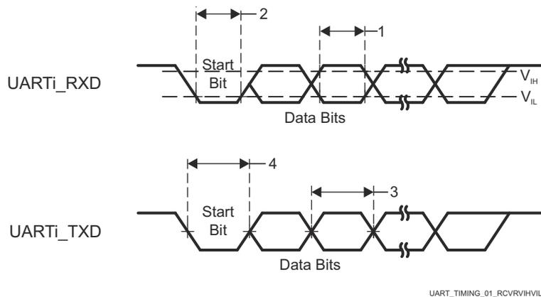
**Figure 6-110. UART Timing Requirements and Switching Characteristics**
