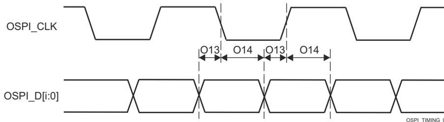
**Figure 6-107. OSPI0 Timing Requirements – Tap DDR, No Loopback**
