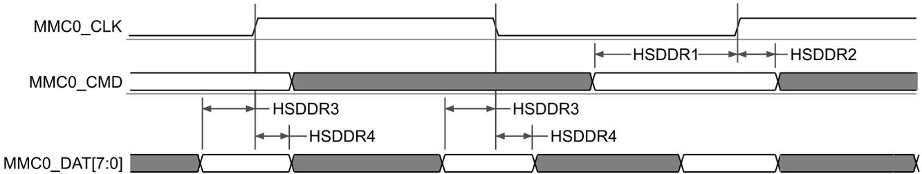
Figure 6-71. MMC0 – High Speed DDR Mode – Receive Mode
