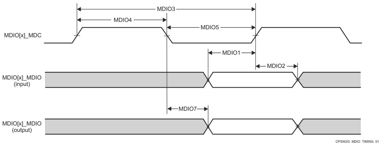
**Figure 6-26. CPSW3G MDIO Timing Requirements and Switching Characteristics**
