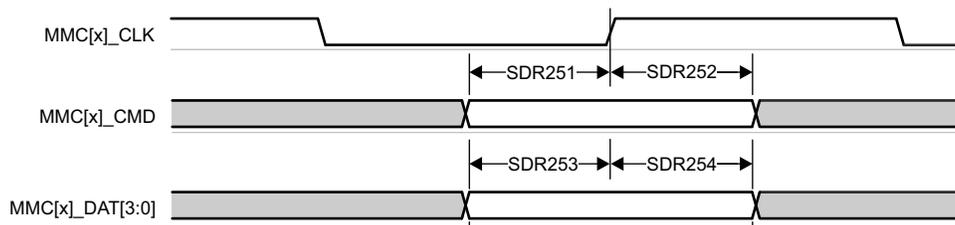
**Figure 6-80. MMC0 – UHS-I SDR25 – Receive Mode**
