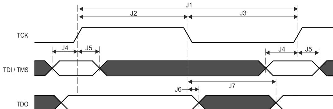
**Figure 6-40. JTAG Timing Requirements and Switching Characteristics**
