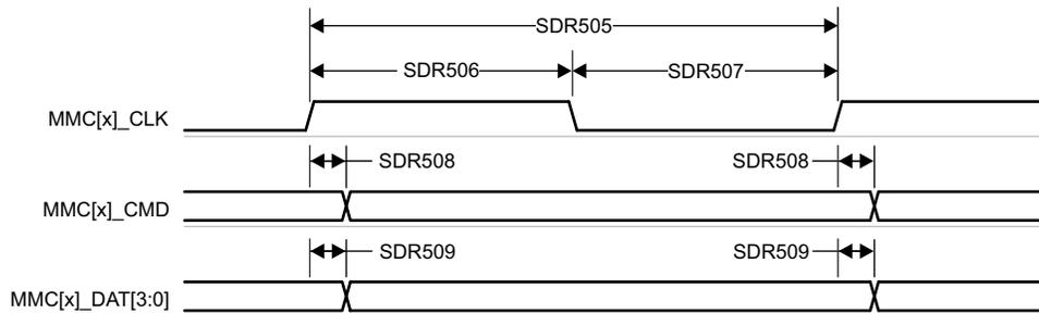
**Figure 6-82. MMC0 – UHS-I SDR50 – Transmit Mode**
