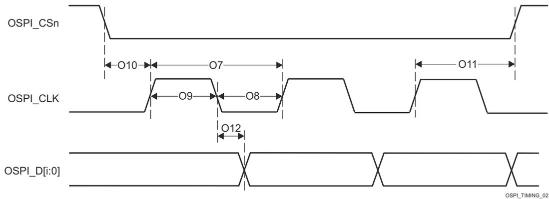
**Figure 6-106. OSPI0 Switching Characteristics – Tap SDR, No Loopback**
