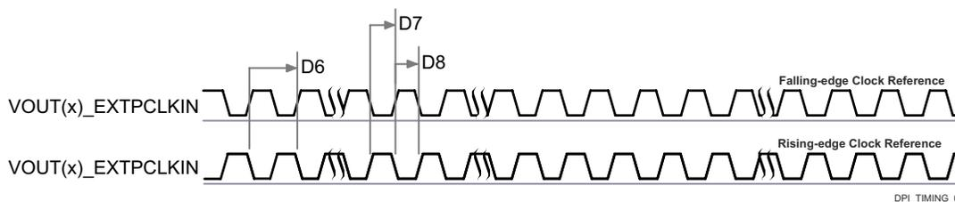
**Figure 6-35. DSS External Pixel Clock Timing Requirements**
