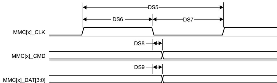
**Figure 6-86. MMC1/MMC2 – Default Speed – Transmit Mode**
