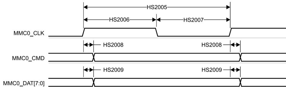
**Figure 6-73. MMC0 – HS200 Mode – Transmit Mode**
