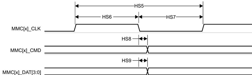
**Figure 6-88. MMC1/MMC2 – High Speed – Transmit Mode**
