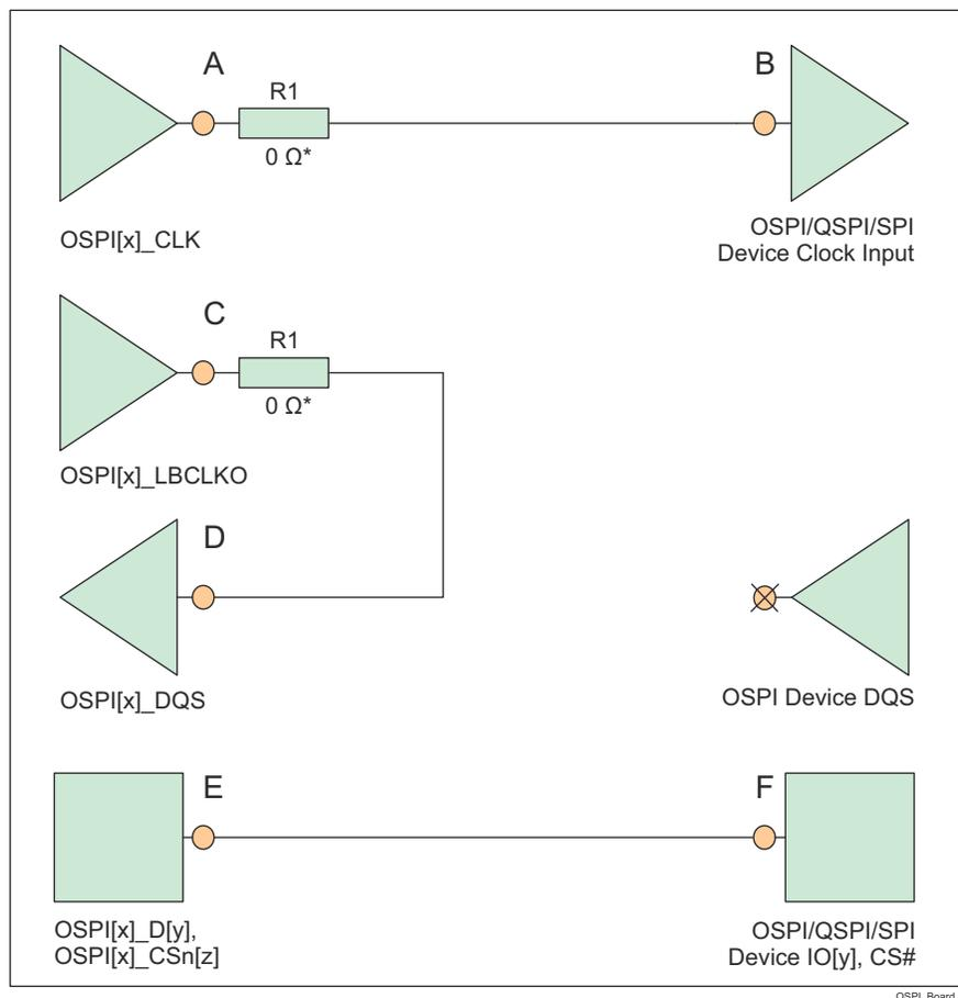
\* 0Ω resistor (R1), located as close as possible to the OSPI[x]\_CLK and OSPI[x]\_LBCLKO pins, is a placeholder for fine tuning, if needed.
