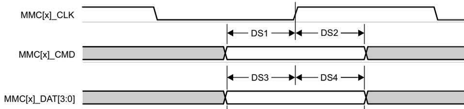
Figure 6-74. MMC0 – Default Speed – Receive Mode
