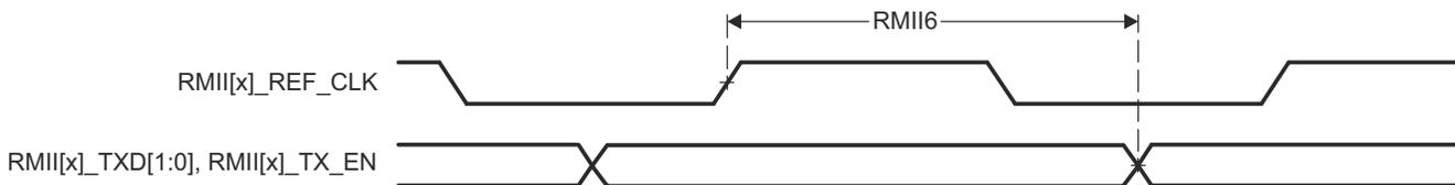
**Figure 6-29. RMII[x]\_TXD[1:0], and RMII[x]\_TX\_EN Switching Characteristics – RMII Mode**
