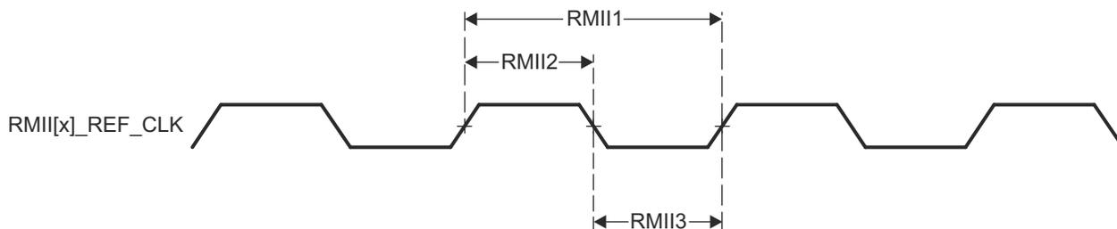
**Figure 6-27. CPSW3G RMII[x]\_REF\_CLK Timing Requirements – RMII Mode**
