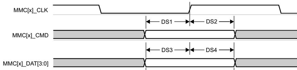
**Figure 6-85. MMC1/MMC2 – Default Speed – Receive Mode**
