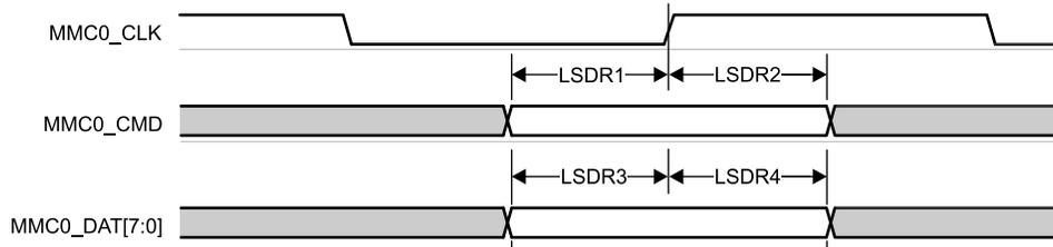
Figure 6-67. MMC0 – Legacy SDR – Receive Mode
