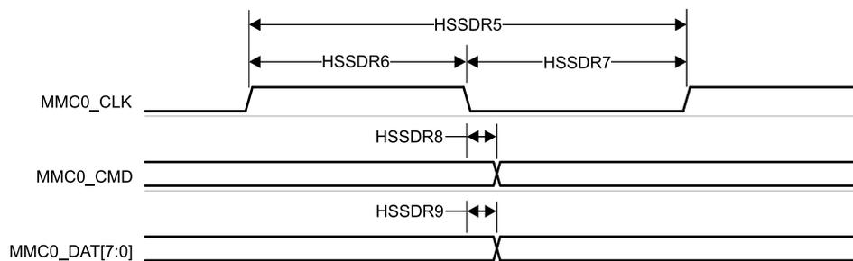
**Figure 6-70. MMC0 – High Speed SDR Mode – Transmit Mode**
