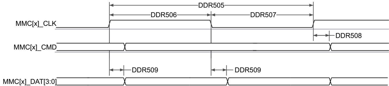
**Figure 6-83. MMC0 – UHS-I DDR50 – Transmit Mode**
