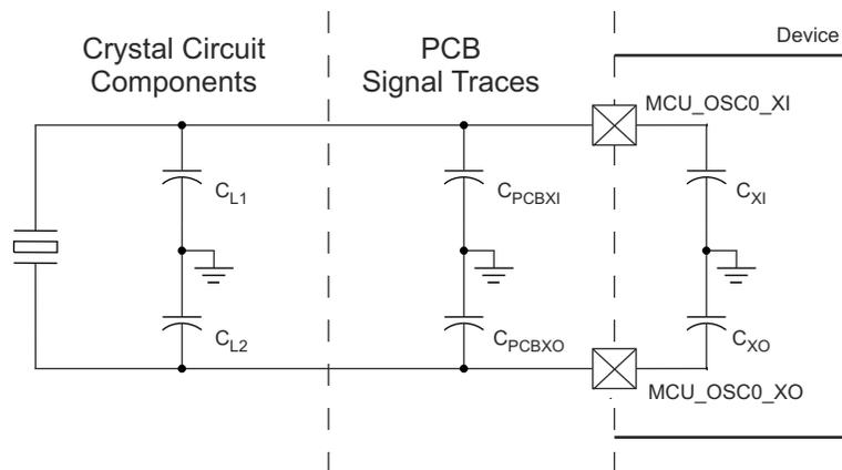
**Figure 6-18. Load Capacitance**
