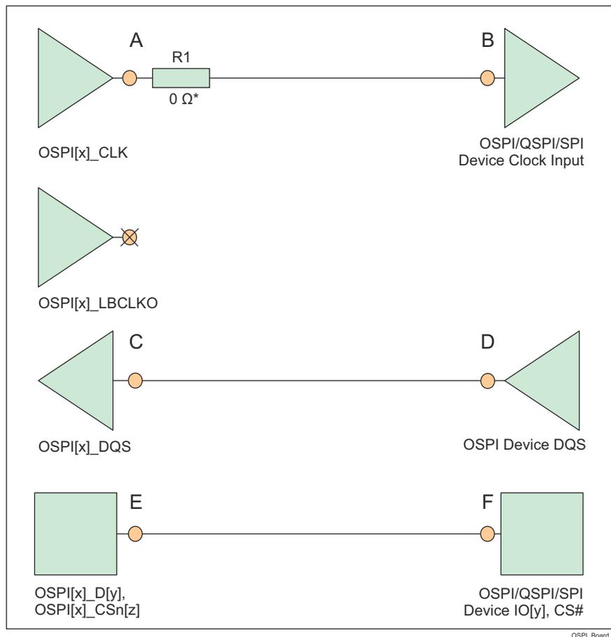
\* 0Ω resistor (R1), located as close as possible to the OSPI[x]\_CLK pin, is a placeholder for fine tuning, if needed.
