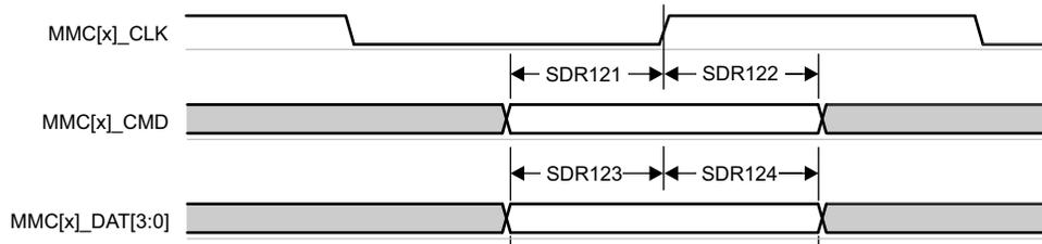
Figure 6-78. MMC0 – UHS-I SDR12 – Receive Mode
