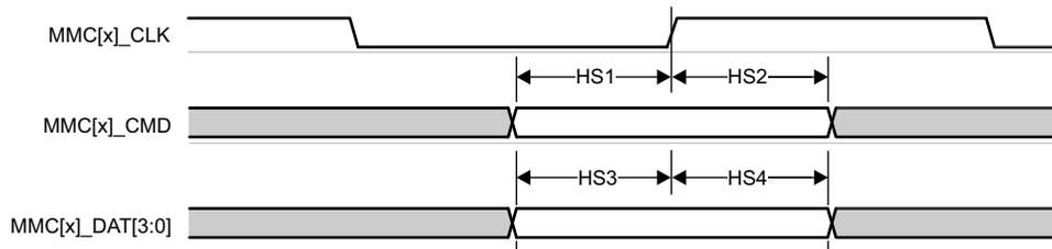
**Figure 6-76. MMC0 – High Speed – Receive Mode**
