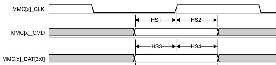
**Figure 6-87. MMC1/MMC2 – High Speed – Receive Mode**
