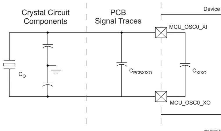
Figure 6-19. Shunt Capacitance
