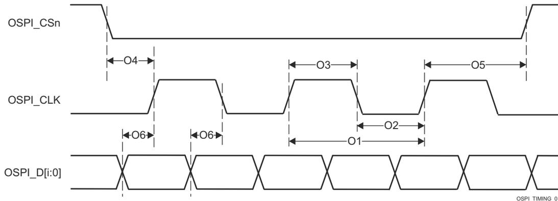
**Figure 6-98. OSPI0 Switching Characteristics – PHY DDR Data Training**
