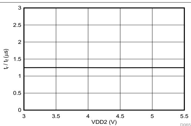
Figure 6-40. Output Rise and Fall Time vs Supply Voltage
