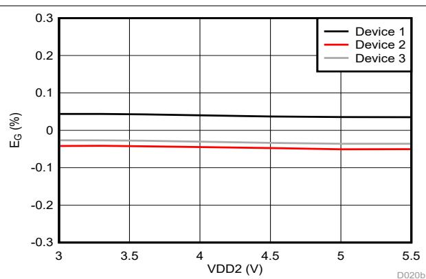
Figure 6-12. Gain Error vs Low-Side Supply Voltage
