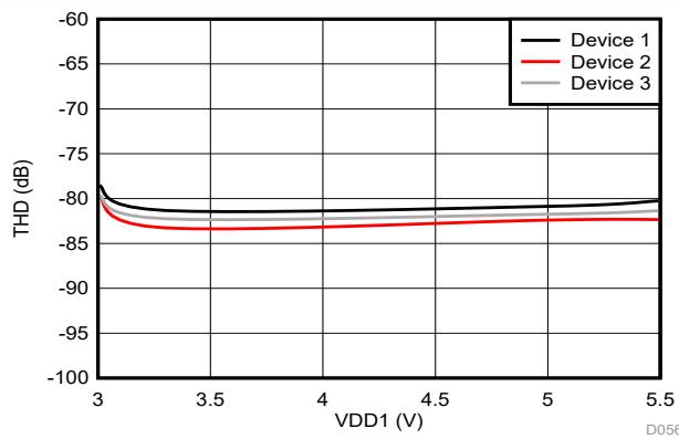
Figure 6-19. Total Harmonic Distortion vs High-Side Supply Voltage
