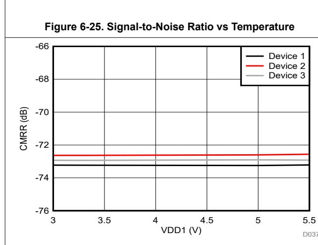
Figure 6-27. Common-Mode Rejection Ratio vs Supply Voltage
