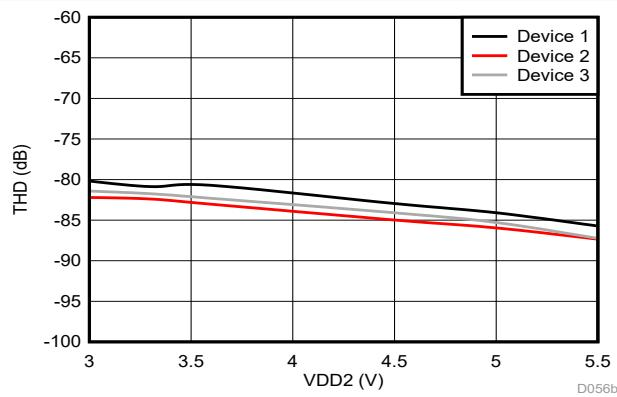
Figure 6-20. Total Harmonic Distortion vs Low-Side Supply Voltage
