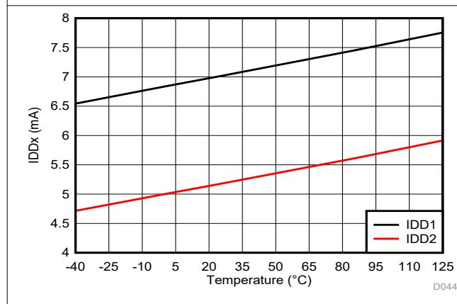
Figure 6-39. Supply Current vs Temperature
