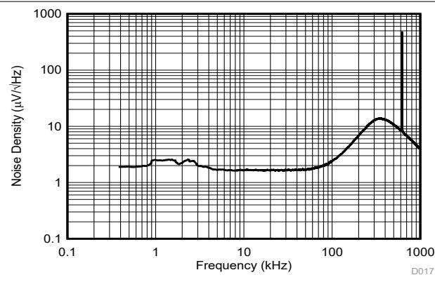
Figure 6-26. Input-Referred Noise Density vs Frequency
