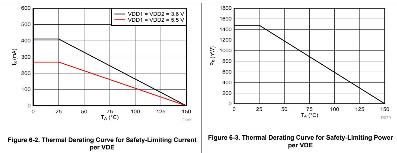
Figure 6-2. Thermal Derating Curve for Safety-Limiting Current per VDE
