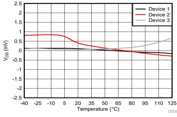
Figure 6-9. Input Offset Voltage vs Temperature
