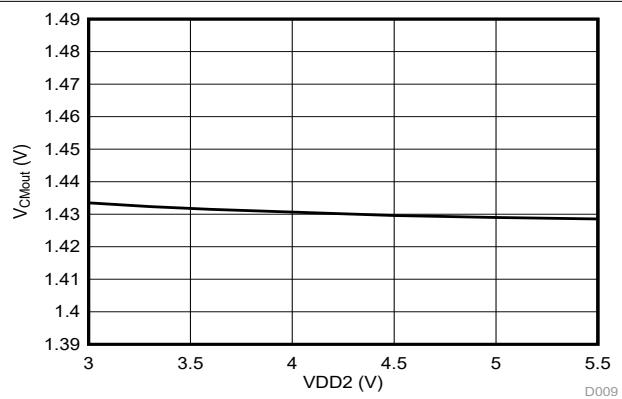
Figure 6-32. Common-Mode Output Voltage vs Supply Voltage
