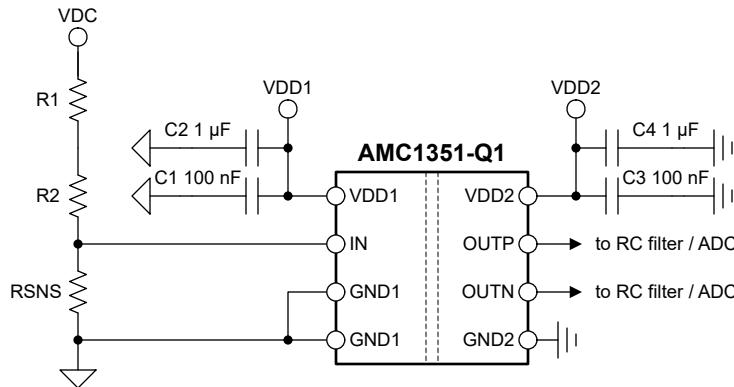
**Figure 9-1. Decoupling of the AMC1351-Q1**
