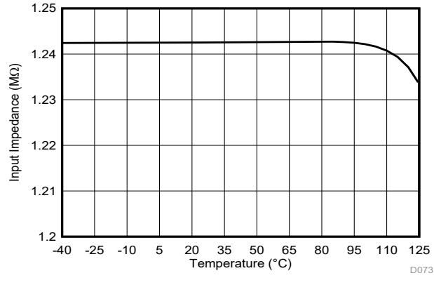
Figure 6-10. Input Impedance vs Temperature
