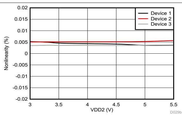
Figure 6-16. Nonlinearity vs Low-Side Supply Voltage
