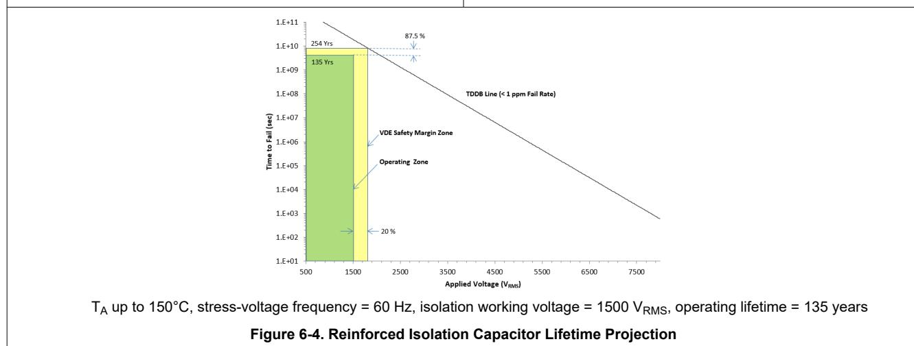
Figure 6-4. Reinforced Isolation Capacitor Lifetime Projection
