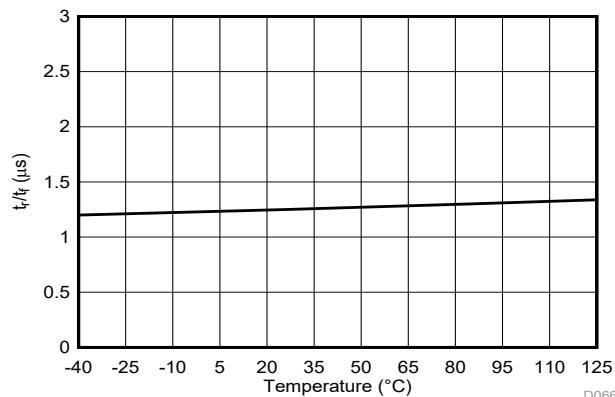
Figure 6-41. Output Rise and Fall Time vs Temperature
