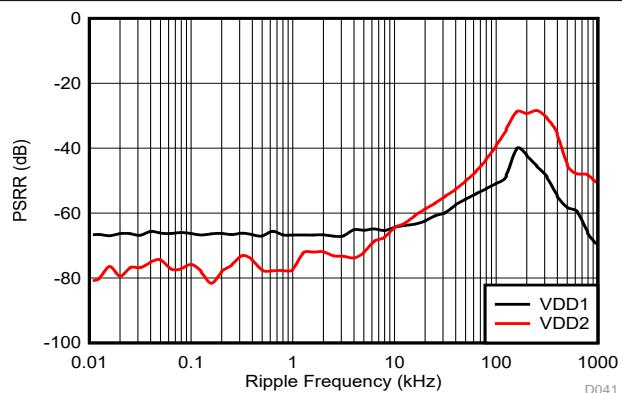
Figure 6-30. Power-Supply Rejection Ratio vs Ripple Frequency
