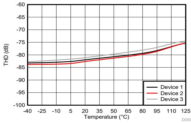
Figure 6-21. Total Harmonic Distortion vs Temperature
