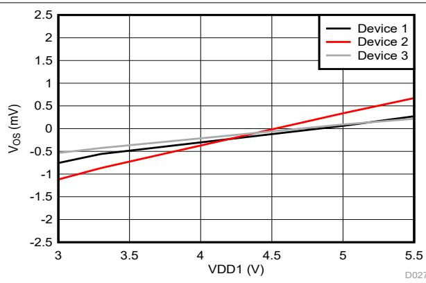
Figure 6-7. Input Offset Voltage vs High-Side Supply Voltage
