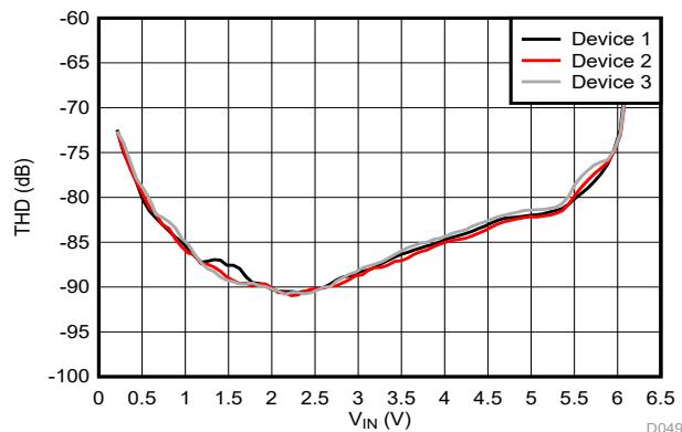
Figure 6-18. Total Harmonic Distortion vs Input Voltage
