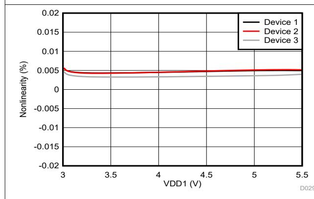
Figure 6-15. Nonlinearity vs High-Side Supply Voltage
