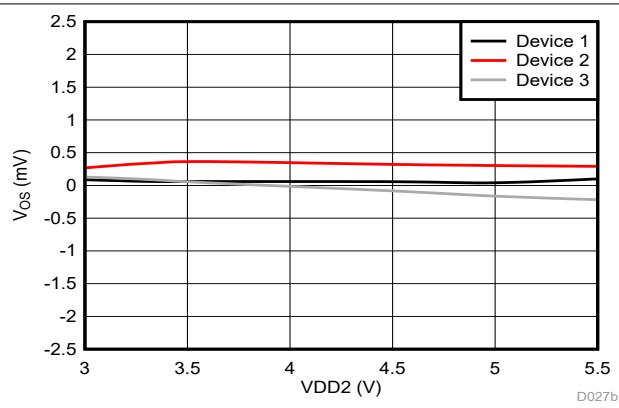
Figure 6-8. Input Offset Voltage vs Low-Side Supply Voltage
