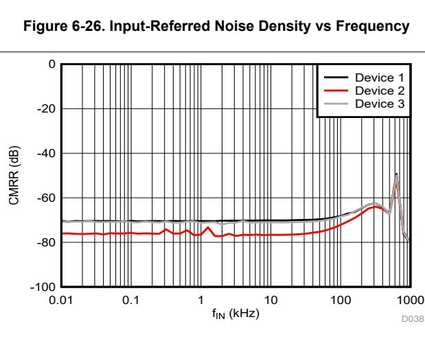
Figure 6-28. Common-Mode Rejection Ratio vs Input Frequency
