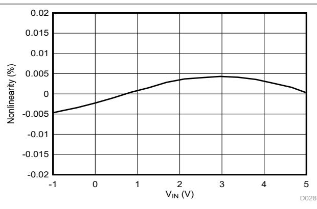
Figure 6-14. Nonlinearity vs Input Voltage
