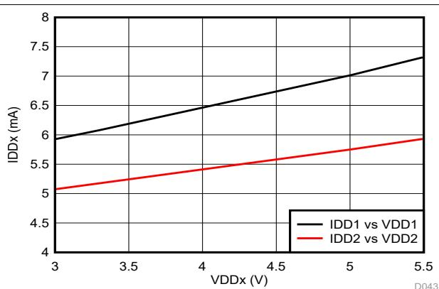
Figure 6-38. Supply Current vs Supply Voltage
