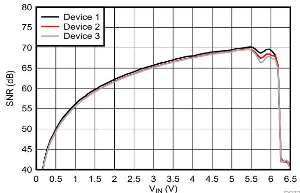
Figure 6-22. Signal-to-Noise Ratio vs Input Voltage
