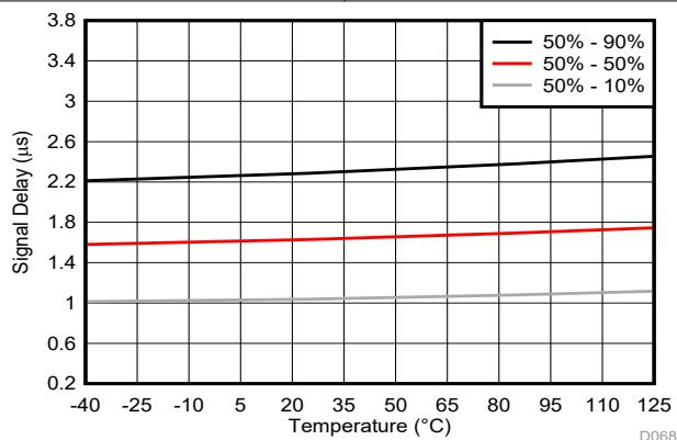
Figure 6-43. Input to Output Signal Delay vs Temperature
