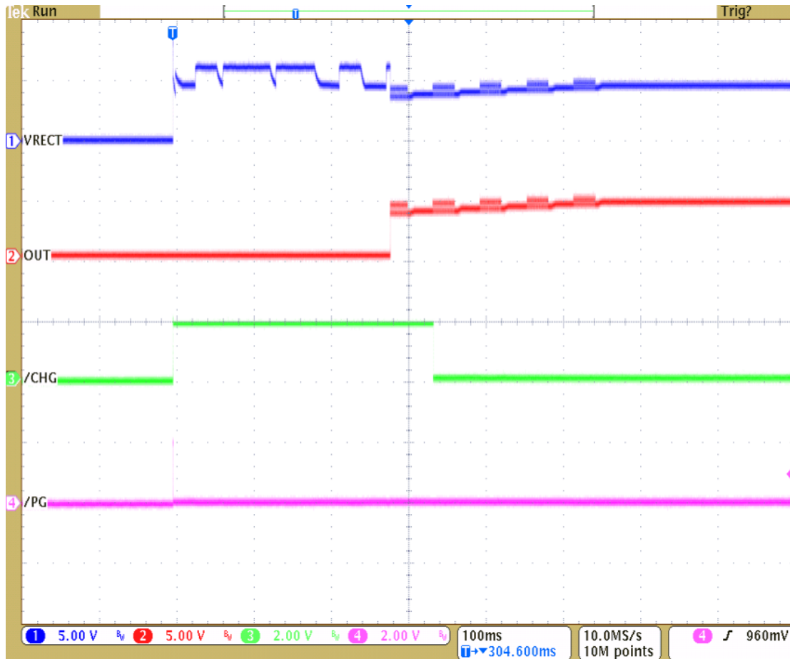
Figure 7-3. Power-Up In a Wireless Power Application
