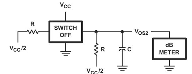
Figure 6-5. Control to Switch Feedthrough Noise Test Circuit
