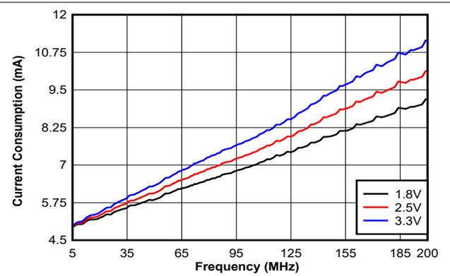
Figure 6-6. Current Consumption vs Frequency and Supply Voltage at 25°C
