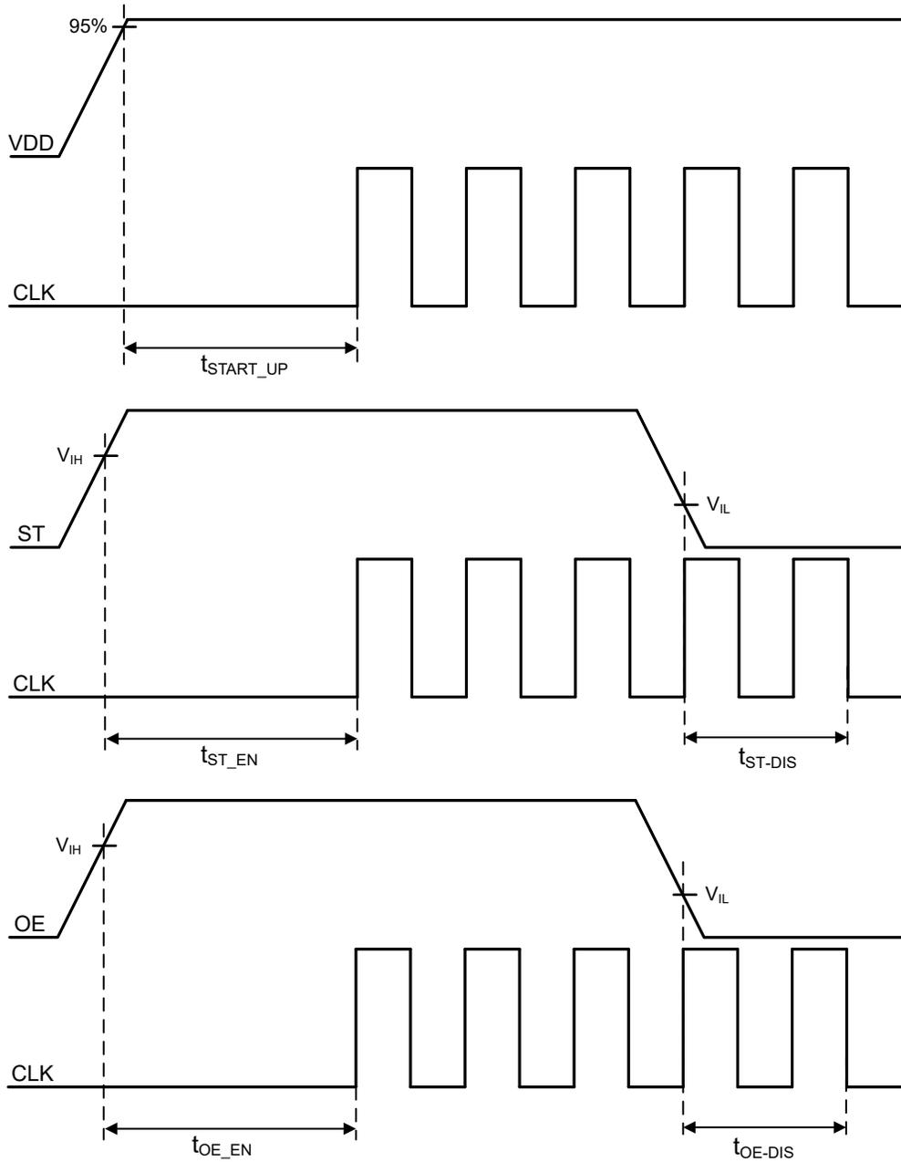
Figure 6-2. Power-On Characteristics
