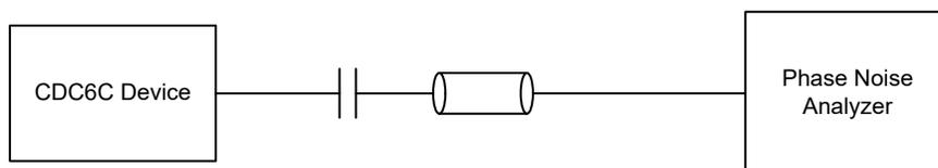
**Figure 7-2. CDC6Cx-Q1 Output Phase Noise Test Configuration**
