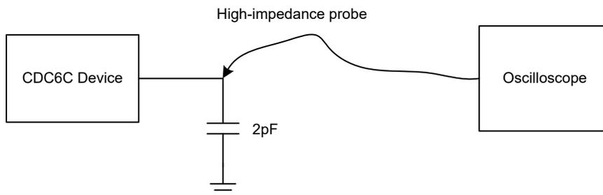
Load capacitor modified based on measurement condition.
