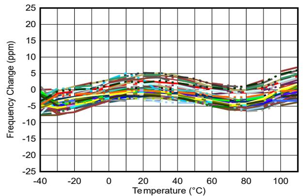
Figure 6-14. Frequency Change vs Temperature at 25MHz and 2.5V Supply, 100 Devices
