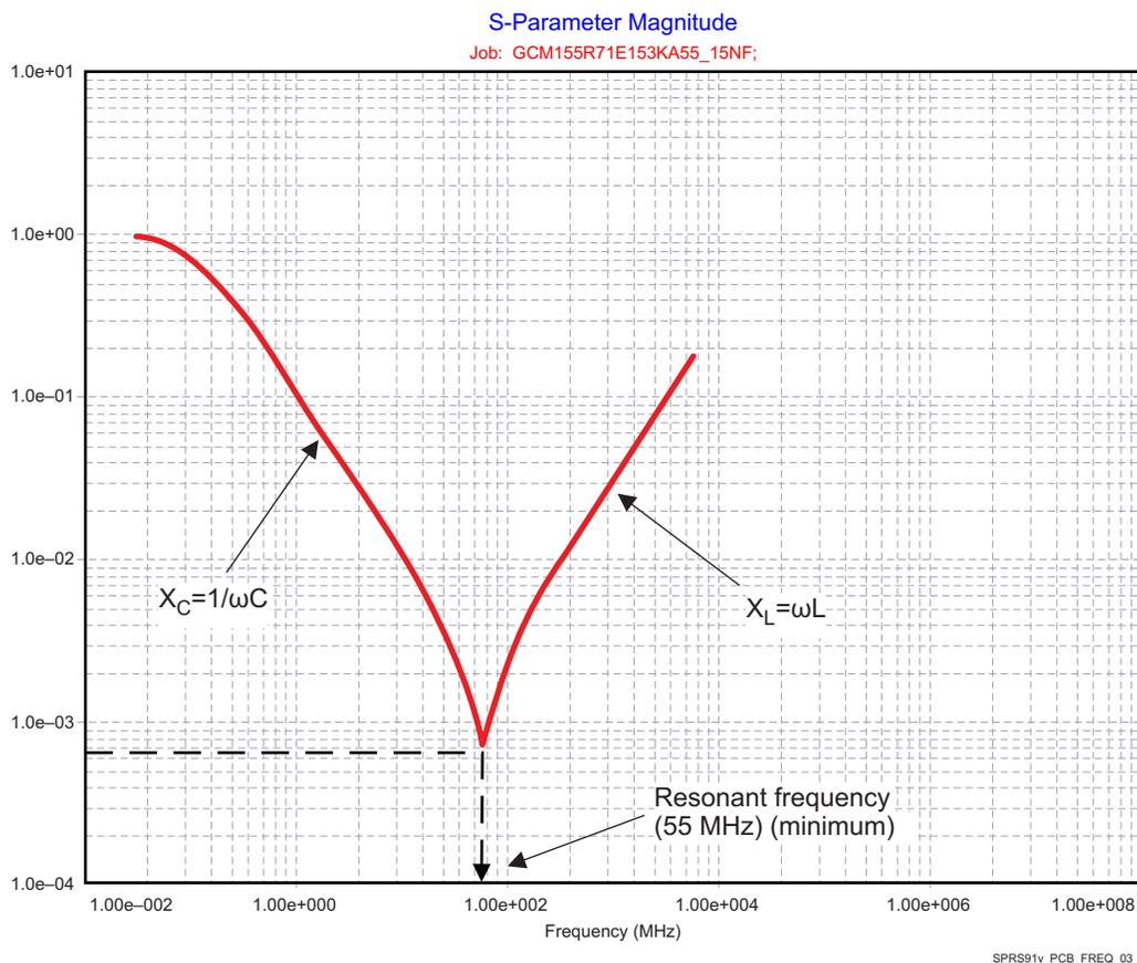
**Figure 7-8. Typical Impedance Profile of a Capacitor**
