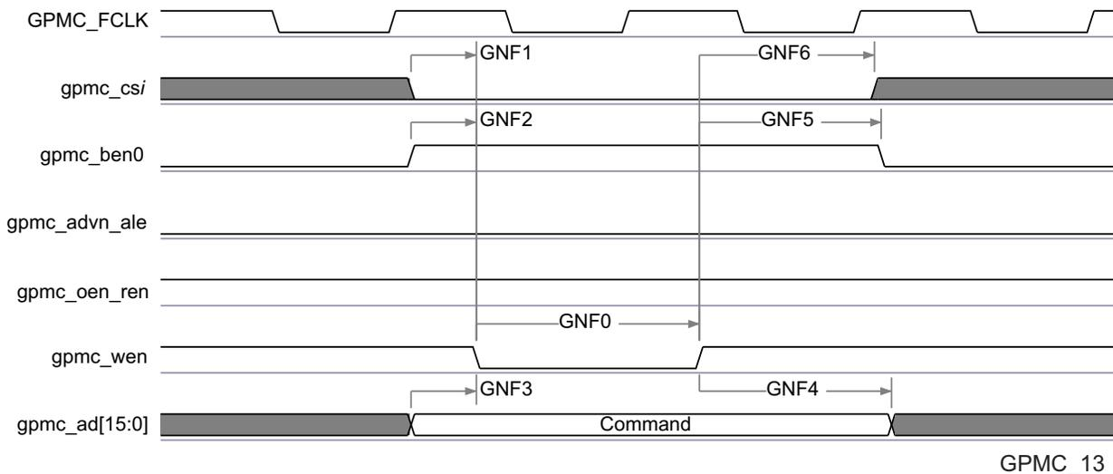
**Figure 5-34. GPMC / NAND Flash - Command Latch Cycle Timing<sup>(1)</sup>**
