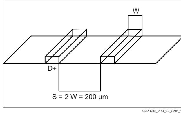
**Figure 7-18. Ground Guard Illustration**
