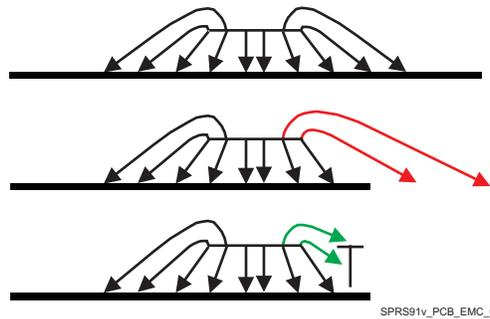
**Figure 7-12. Field Lines of a Signal Above Ground**
