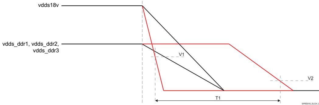
**Figure 5-7. vdds18v and vdds\_dds\* Discharge Relationship<sup>(1)</sup>**
