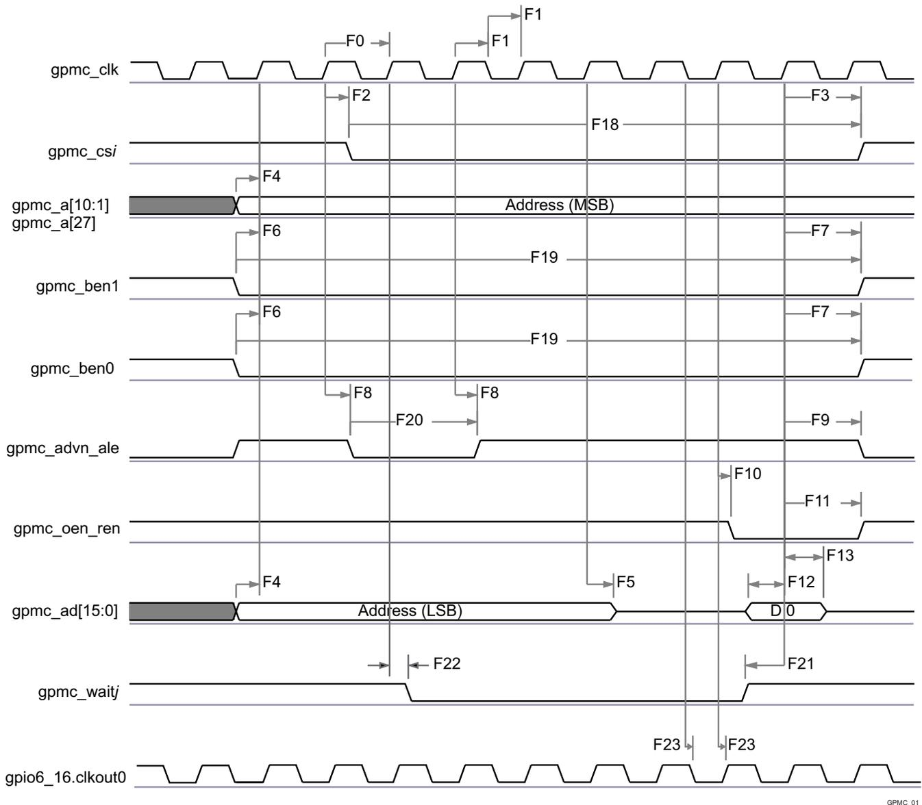
Figure 5-22. GPMC / Multiplexed 16bits NOR Flash - Synchronous Single Read - (GpmcFCLKDivider = 0)<sup>(1)(2)</sup>
