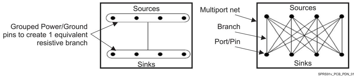
Figure 7-5. Pin-grouping concept: Lumped and Distributed Methodologies
