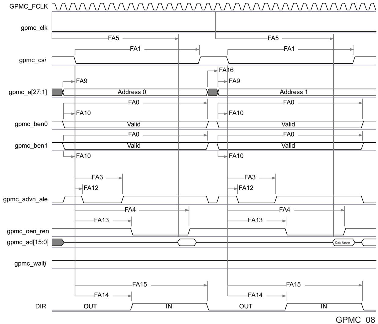
**Figure 5-29. GPMC / NOR Flash - Asynchronous Read - 32-bit Timing<sup>(1)(2)(3)</sup>**
