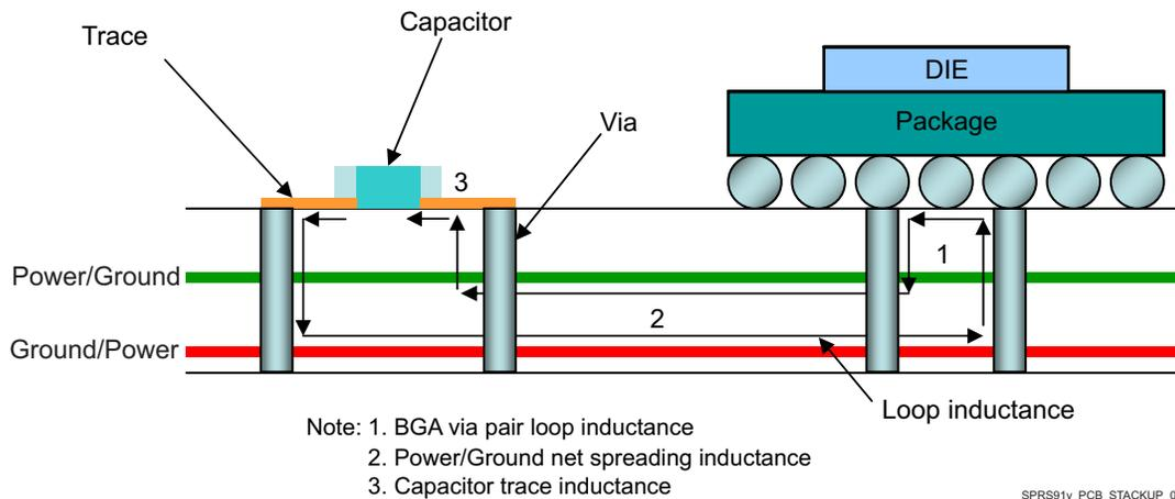
**Figure 7-1. Minimize Loop Inductance With Proper Layer Assignment**
