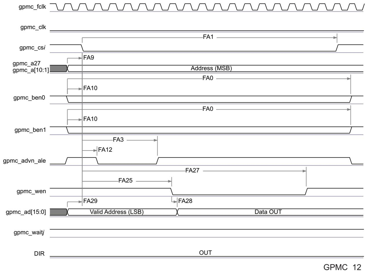
**Figure 5-33. GPMC / Multiplexed NOR Flash - Asynchronous Write - Single Word Timing<sup>(1)</sup>**
