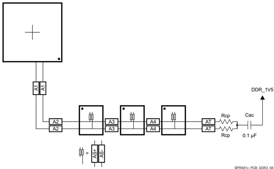
Figure 7-37. CK Routing for Three Single-Side DDR3 Devices
