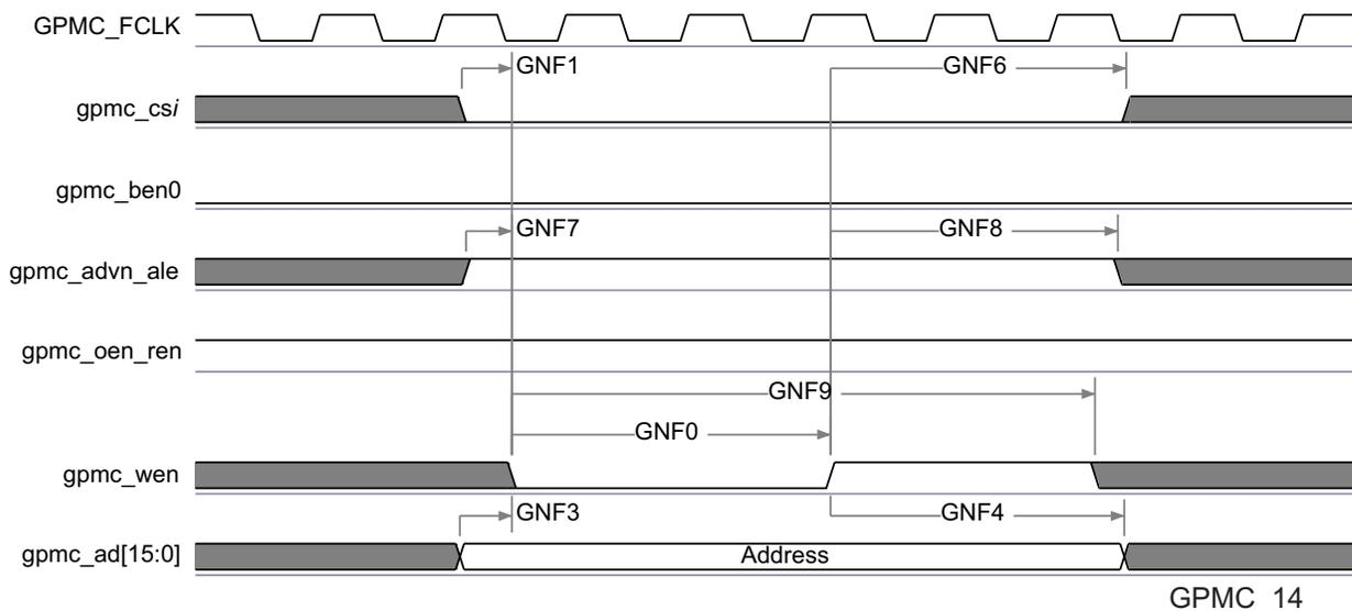
**Figure 5-35. GPMC / NAND Flash - Address Latch Cycle Timing<sup>(1)</sup>**
