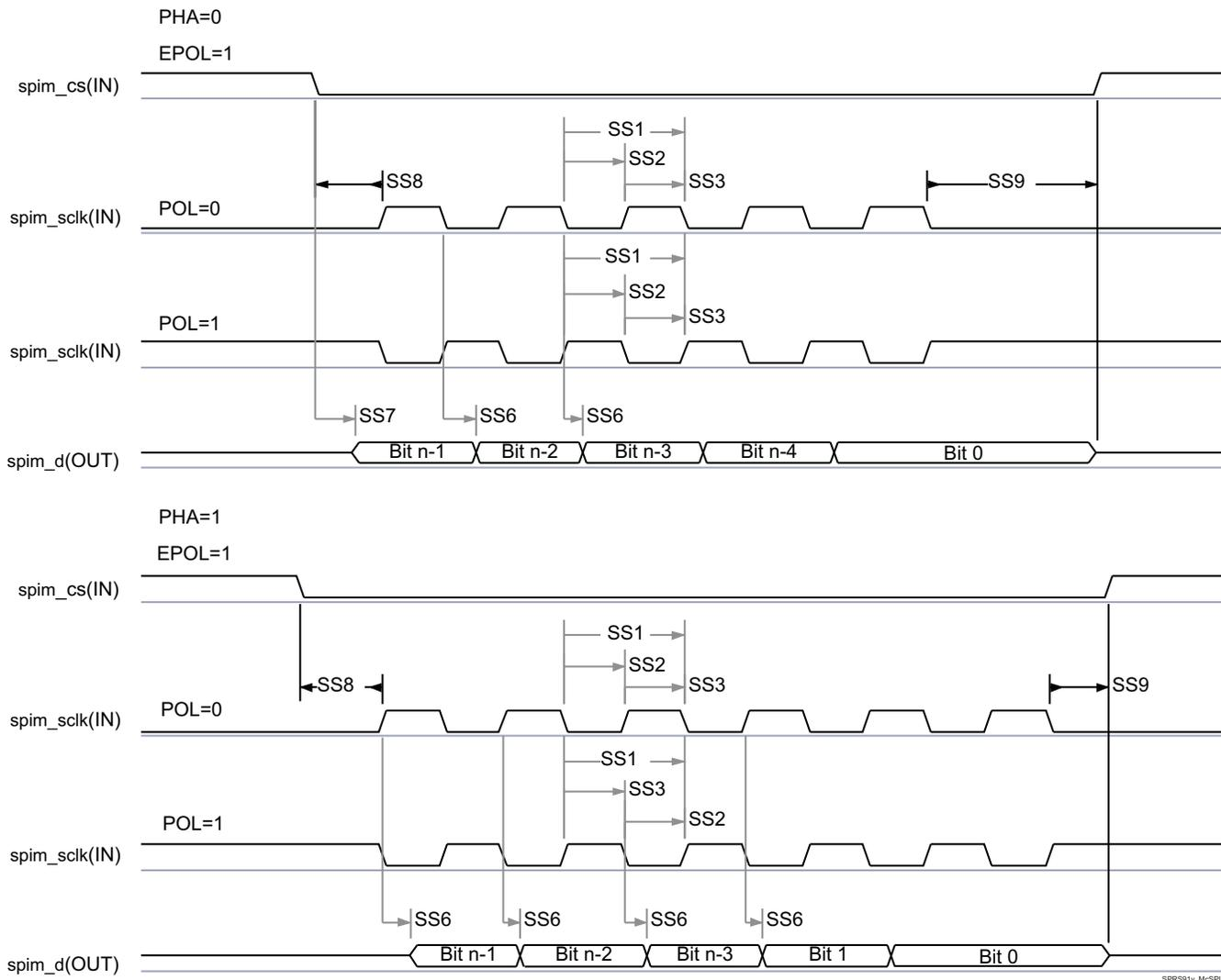
Figure 5-43. McSPI - Slave Mode Transmit
