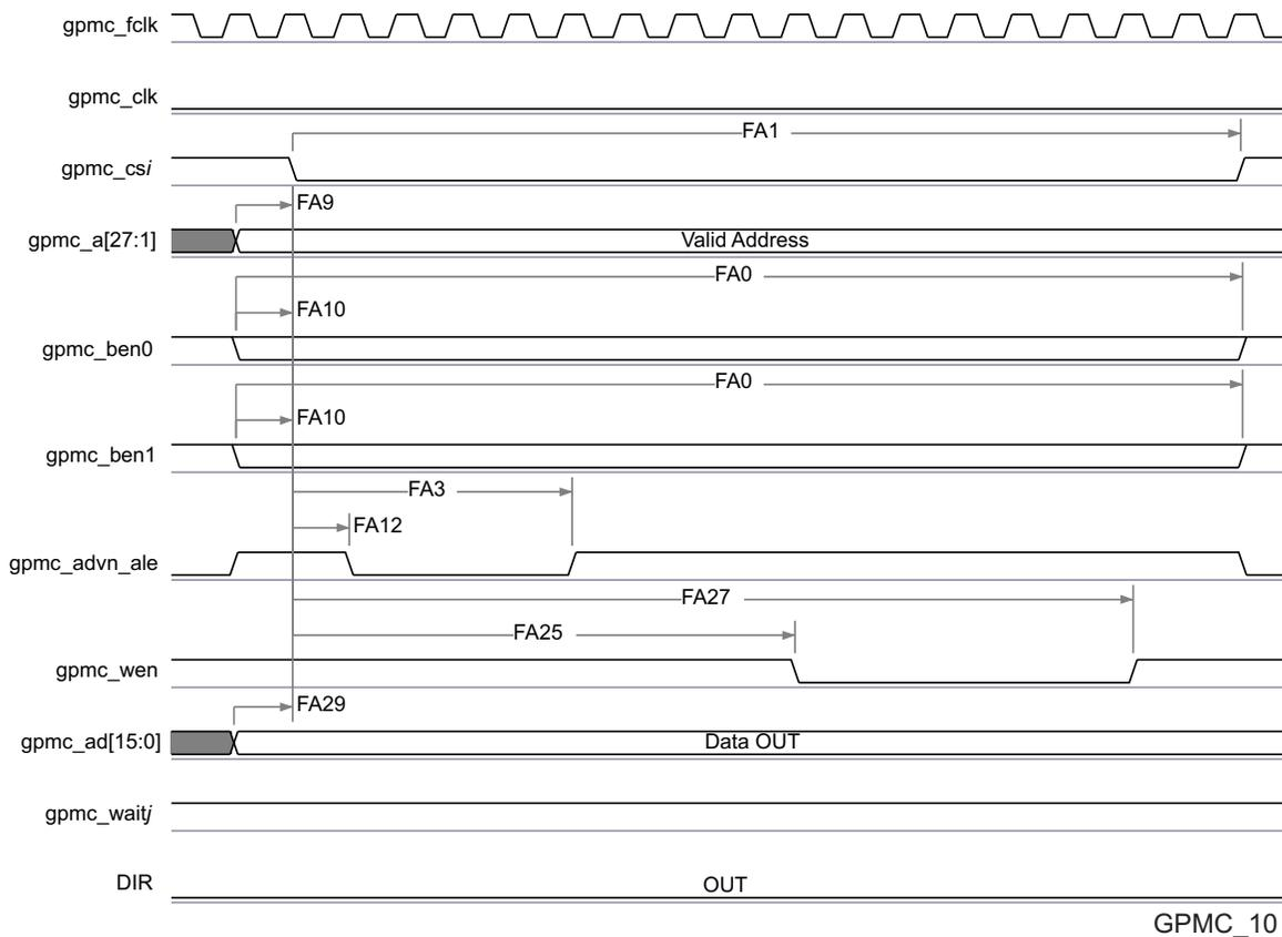
**Figure 5-31. GPMC / NOR Flash - Asynchronous Write - Single Word Timing<sup>(1)</sup>**
