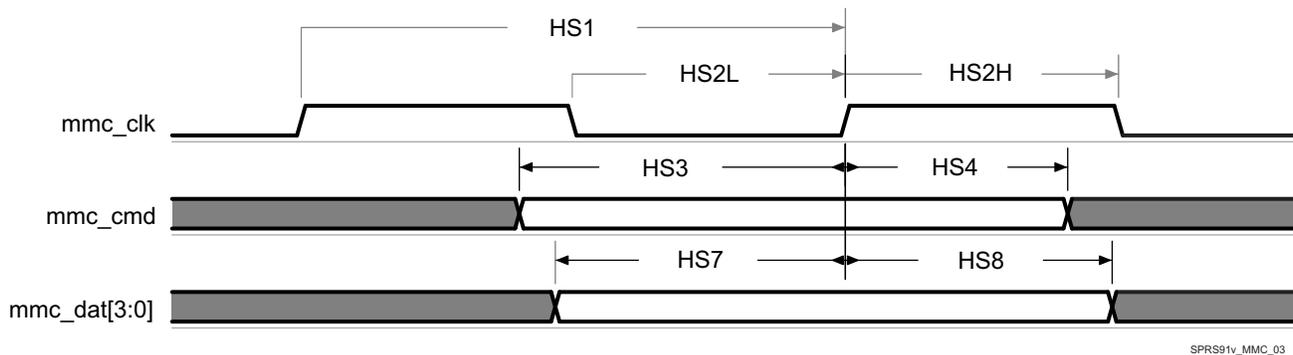
**Figure 5-56. MMC/SD/SDIOj in - High Speed - Receiver Mode**
