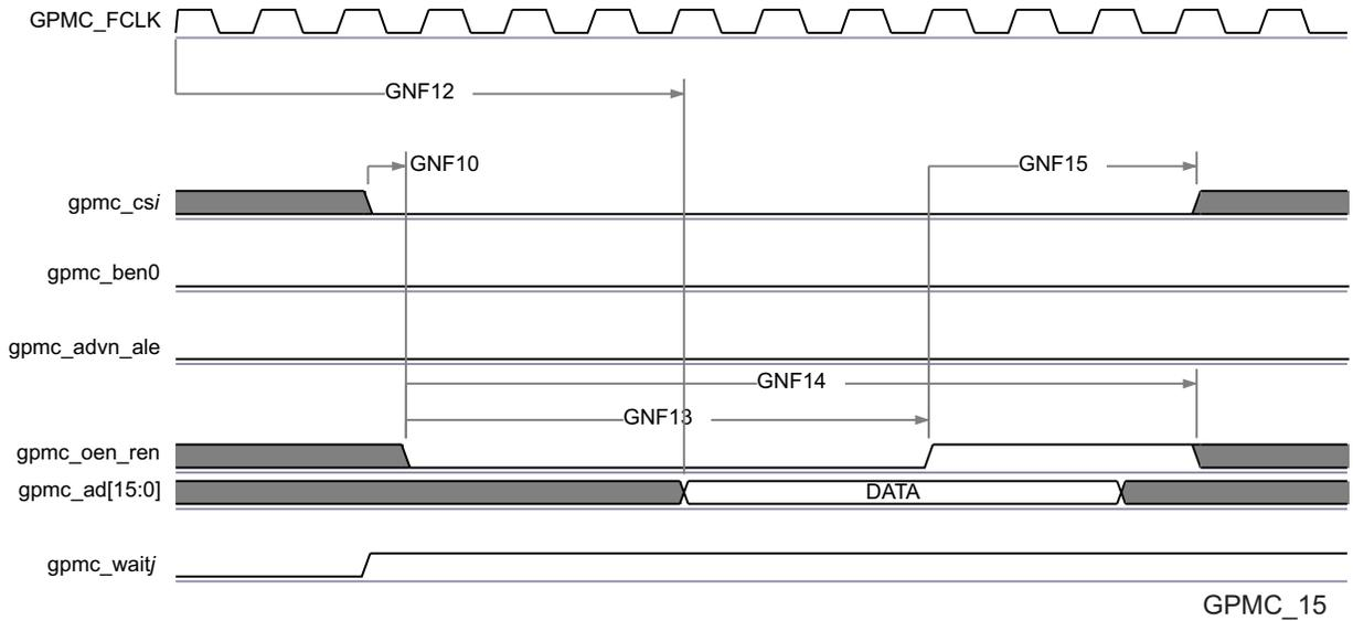
**Figure 5-36. GPMC / NAND Flash - Data Read Cycle Timing<sup>(1)(2)(3)</sup>**
