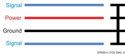
**Figure 7-13. Guard Ring Routing**
