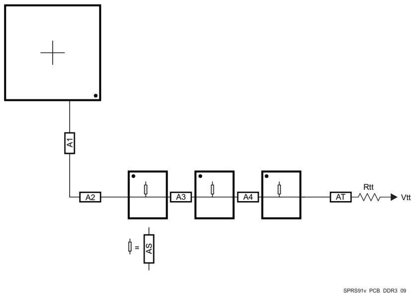
Figure 7-38. ADDR\_CTRL Routing for Three Single-Side DDR3 Devices
