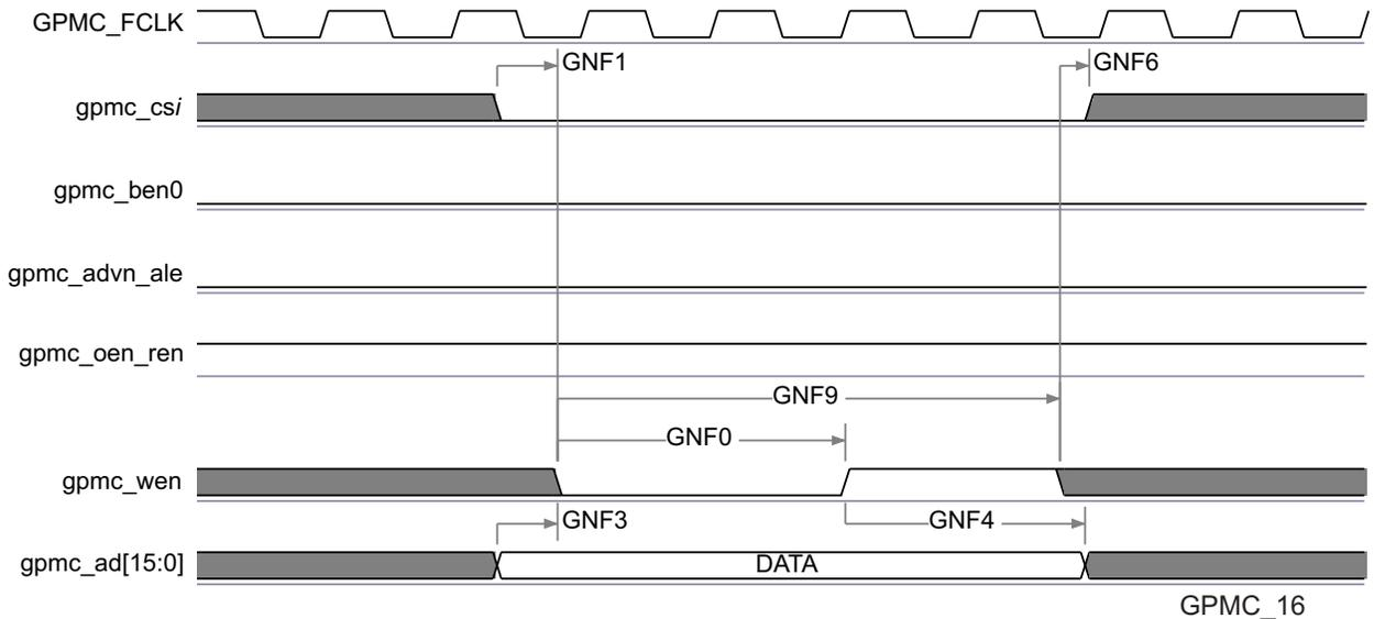
**Figure 5-37. GPMC / NAND Flash - Data Write Cycle Timing<sup>(1)</sup>**
