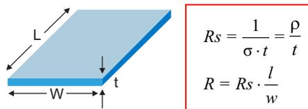
Figure 7-3. Depiction of Sheet Resistivity and Resistance
