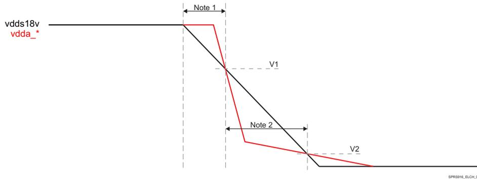
**Figure 5-8. vdds18v and vdda\_\* Discharge Relationship<sup>(3)</sup>**
