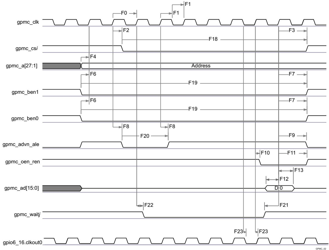
**Figure 5-23. GPMC / Non-Multiplexed 16bits NOR Flash - Synchronous Single Read - (GpmcFCLKDivider = 0)<sup>(1)(2)</sup>**
