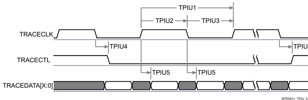
**Figure 5-65. TPIU—PLL DDR Transmit Mode<sup>(1)</sup>**
