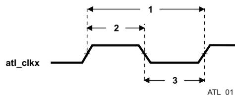
**Figure 5-62. ATL\_CLKOUTx Timing**
