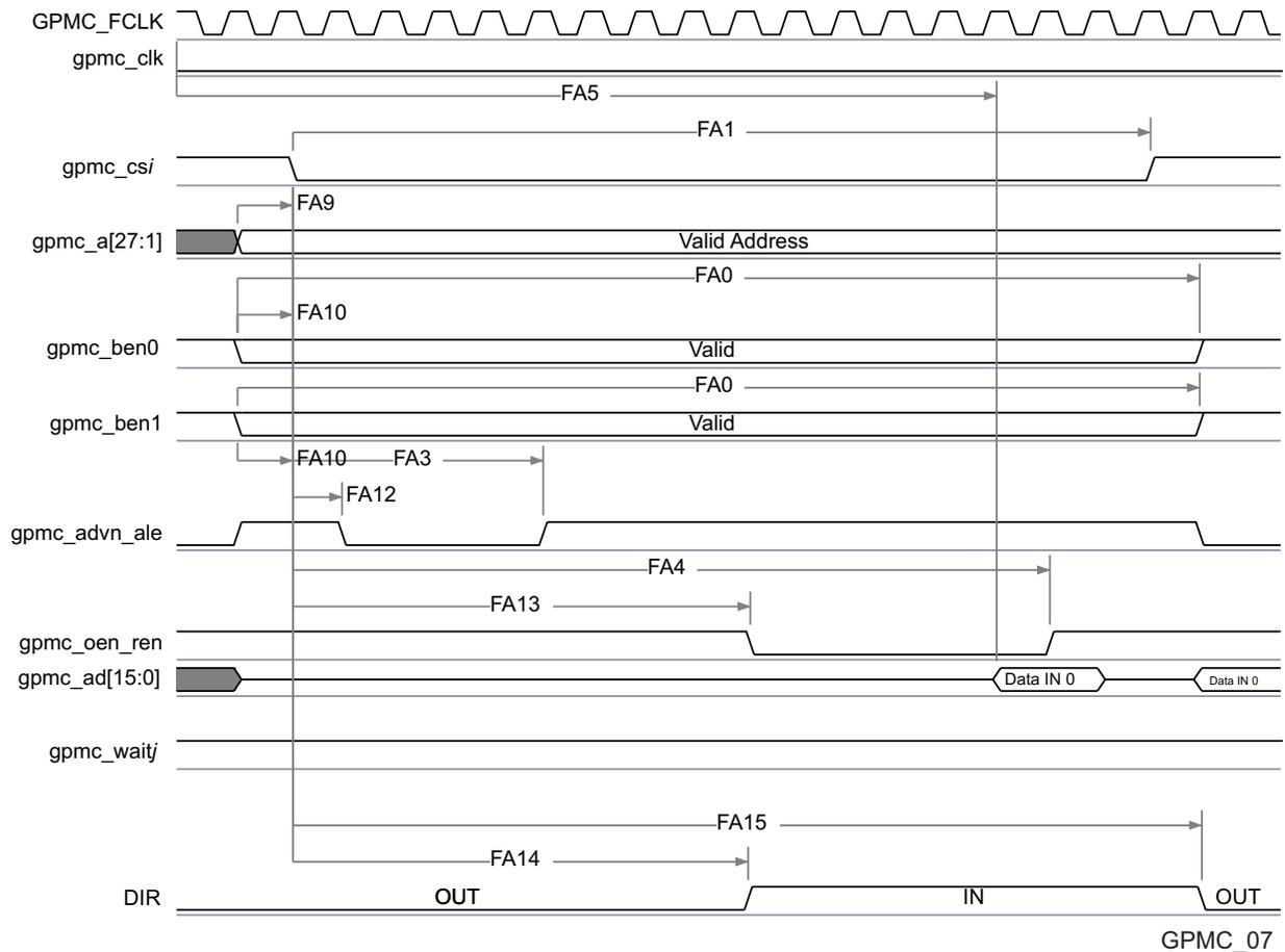
**Figure 5-28. GPMC / NOR Flash - Asynchronous Read - Single Word Timing<sup>(1)(2)(3)</sup>**
