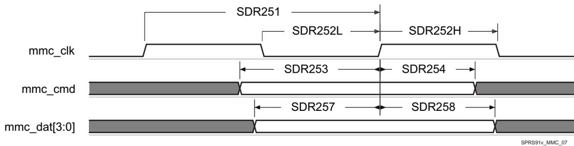
**Figure 5-60. MMC/SD/SDIOj in - SDR25 - Receiver Mode**
