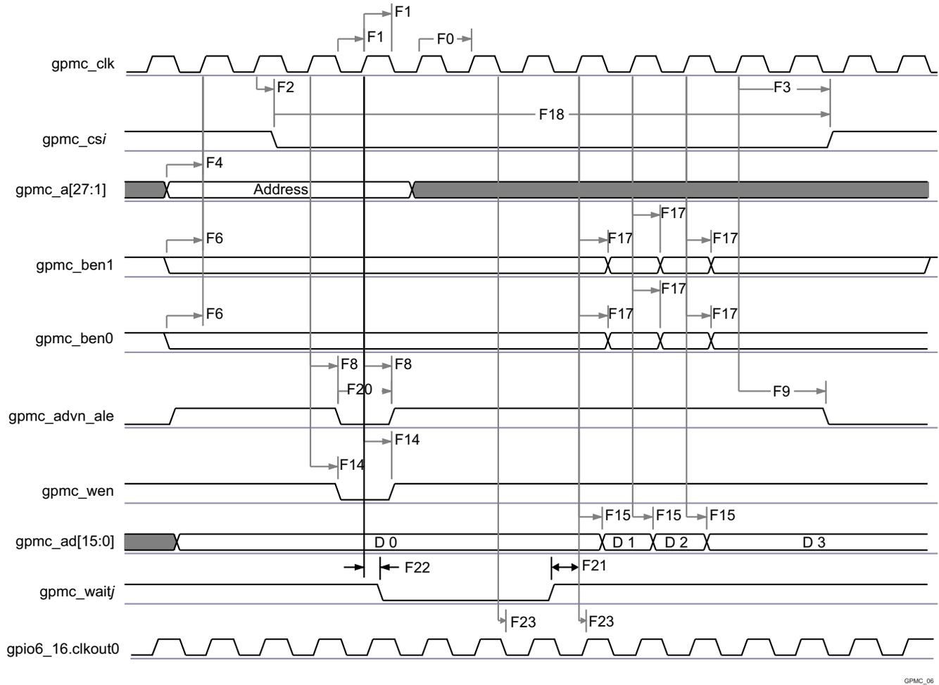
**Figure 5-27. GPMC / Non-Multiplexed 16bits NOR Flash - Synchronous Burst Write 4x16bits - (GpmcFCLKDivider = 0)<sup>(1)(2)</sup>**
