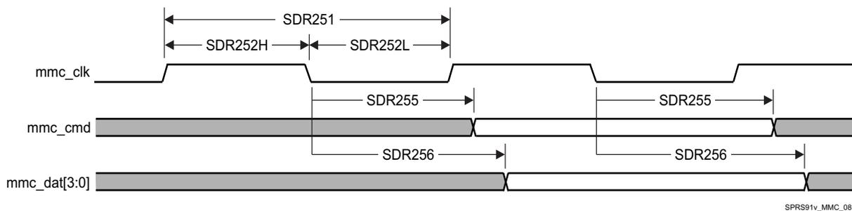
**Figure 5-61. MMC/SD/SDIOj in - SDR25 - Transmitter Mode**
