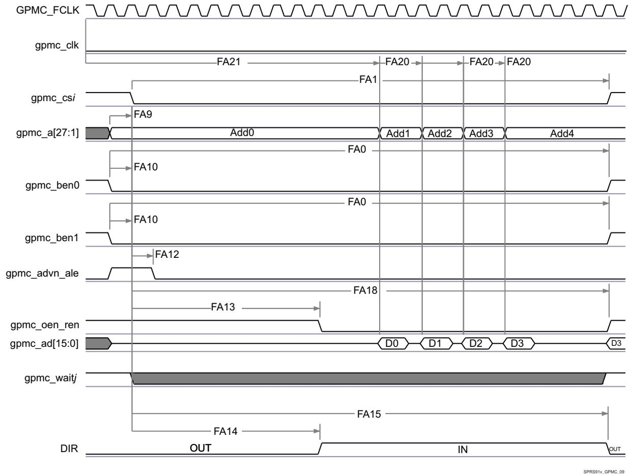
**Figure 5-30. GPMC / NOR Flash - Asynchronous Read - Page Mode 4x16-bit Timing<sup>(1)(2)(3)(4)</sup>**
