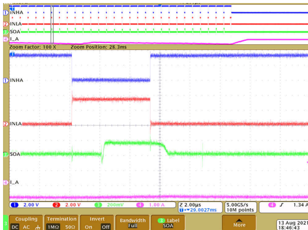
Figure 9-6. Driver PWM operation with feedback
