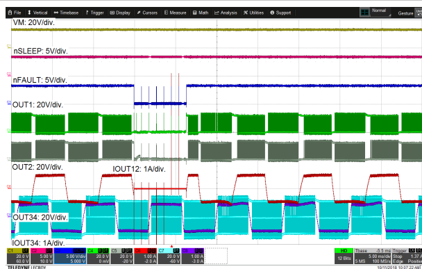
Figure 8-15. Over Current Protection and Recovery
