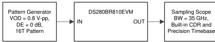
Figure 23. FIR Test Setup
