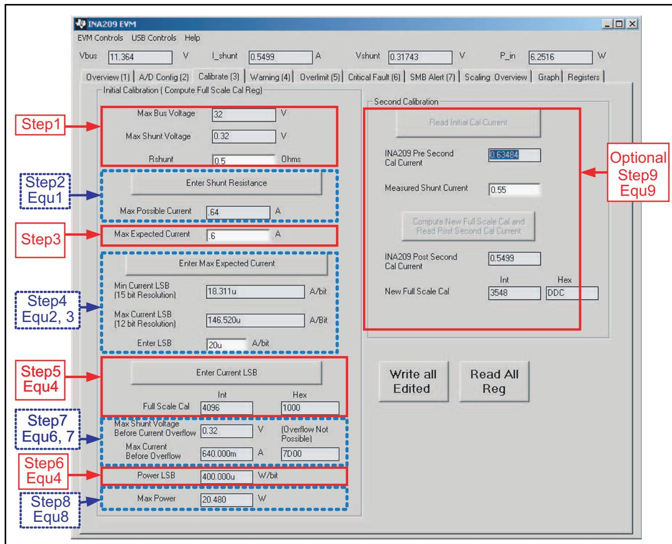
Figure 25. INA209 Calibration Software Automatically Computes Calibration Steps 1-9
