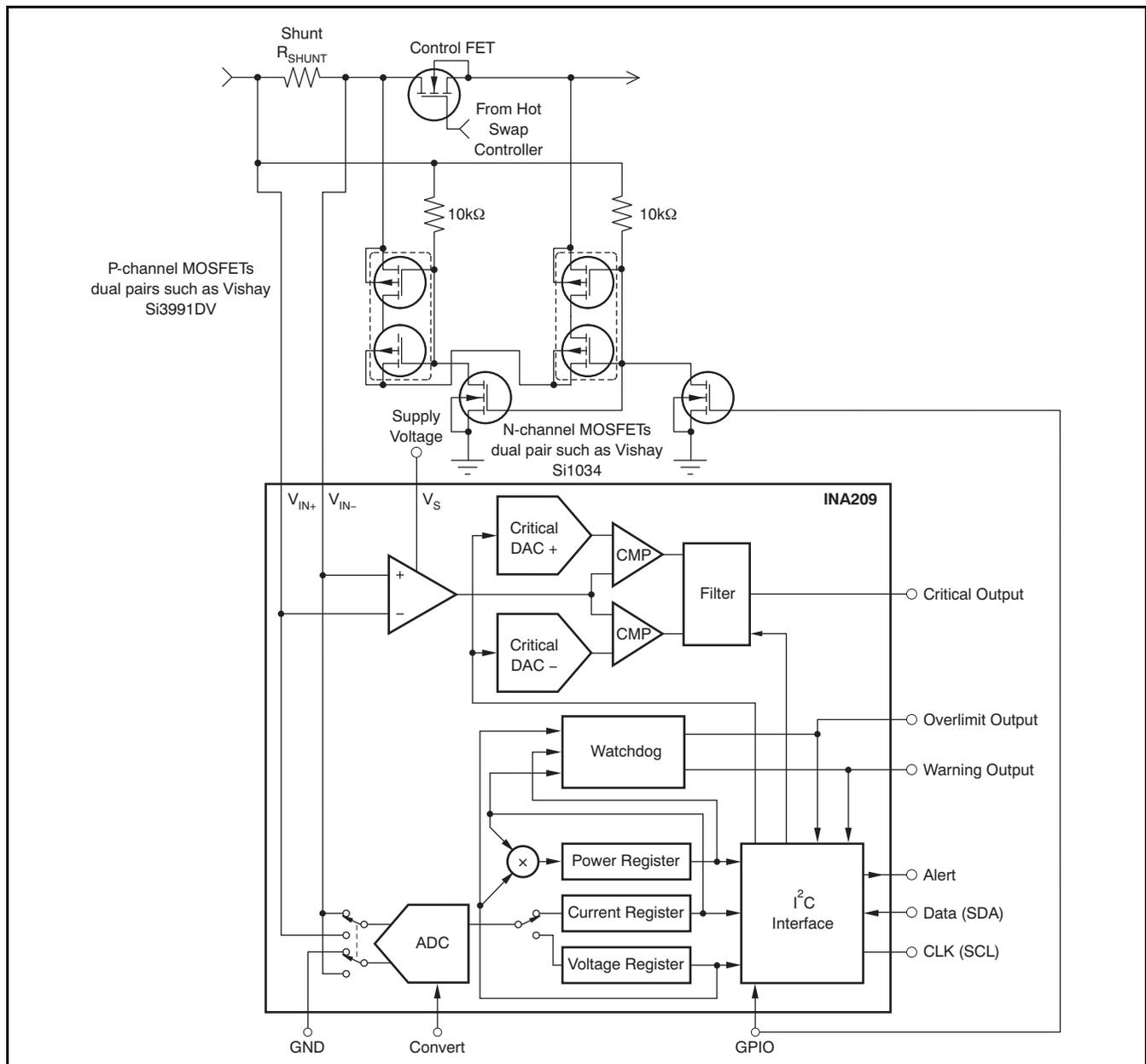
Figure 24. External Circuitry for Additional  $V_{BUS}$  Input
