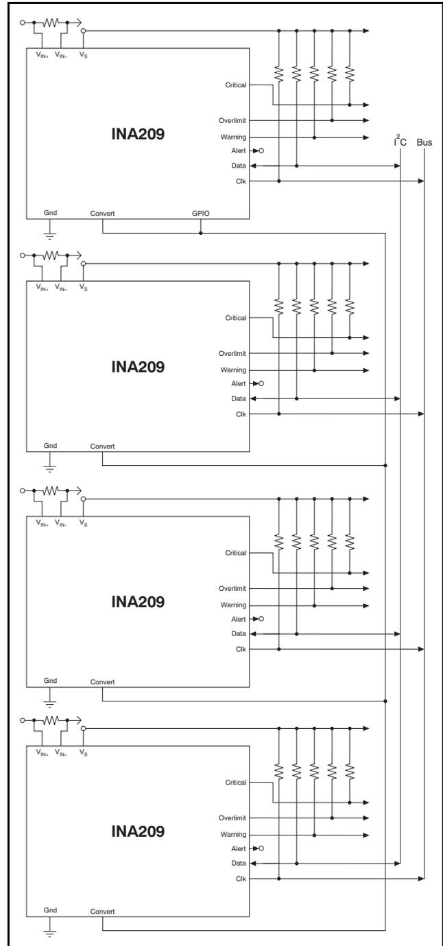
**Figure 23. Multichannel Data Acquisition with Simultaneous Sampling**
