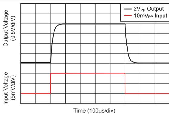
Figure 5-17. Step Response (10-mV<sub>PP</sub> Input Step)
