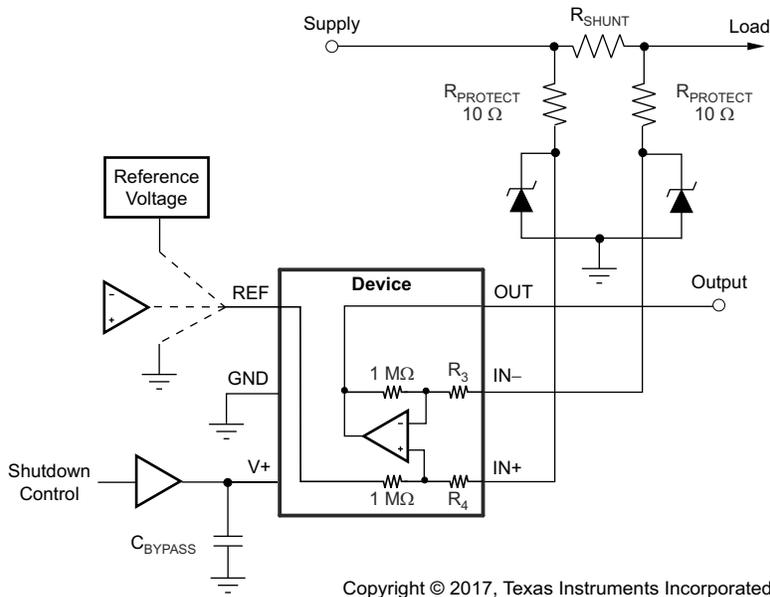
**Figure 6-5. INA21x Transient Protection Using Dual Zener Diodes**
