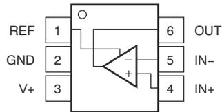
**Figure 4-1. DCK Package 6-Pin SC70 Top View**
