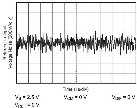
Figure 5-16. 0.1-Hz to 10-Hz Voltage Noise (Referred-To-Input)
