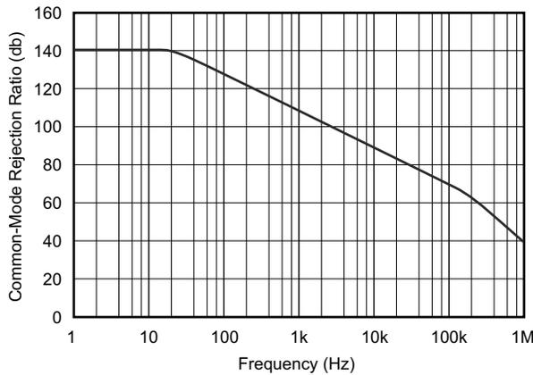
$V_S = 5\text{ V}$        $V_{CM} = 1\text{ V sine}$        $V_{DIF} = \text{shorted}$
