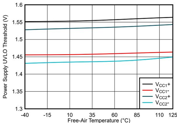
**Figure 6-11. Power Supply Undervoltage Threshold vs Free-Air Temperature**
