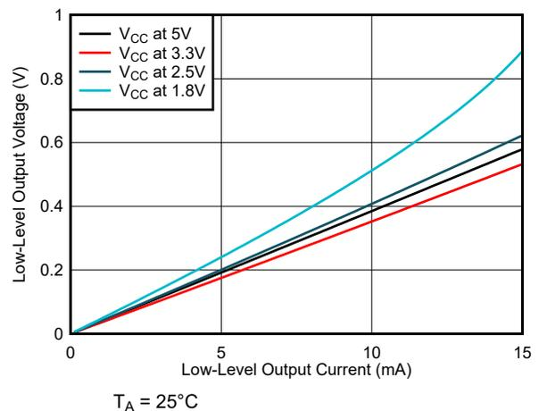
**Figure 6-10. Low-Level Output Voltage vs Low-Level Output Current**
