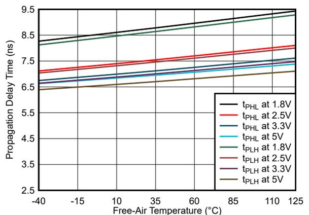
Figure 6-12. Propagation Delay Time vs Free-Air Temperature
