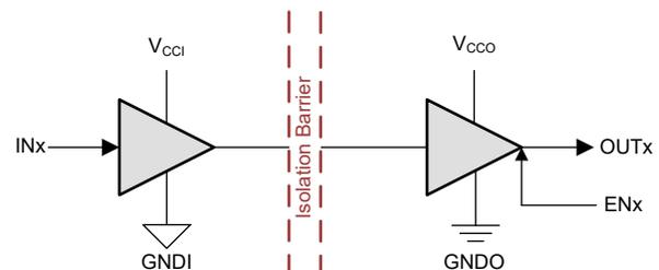
V<sub>CCI</sub>=Input supply, V<sub>CCO</sub>=Output supply
