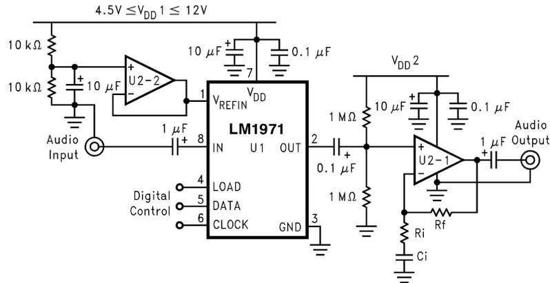
Figure 20. Active Reference with Active Gain Buffering
