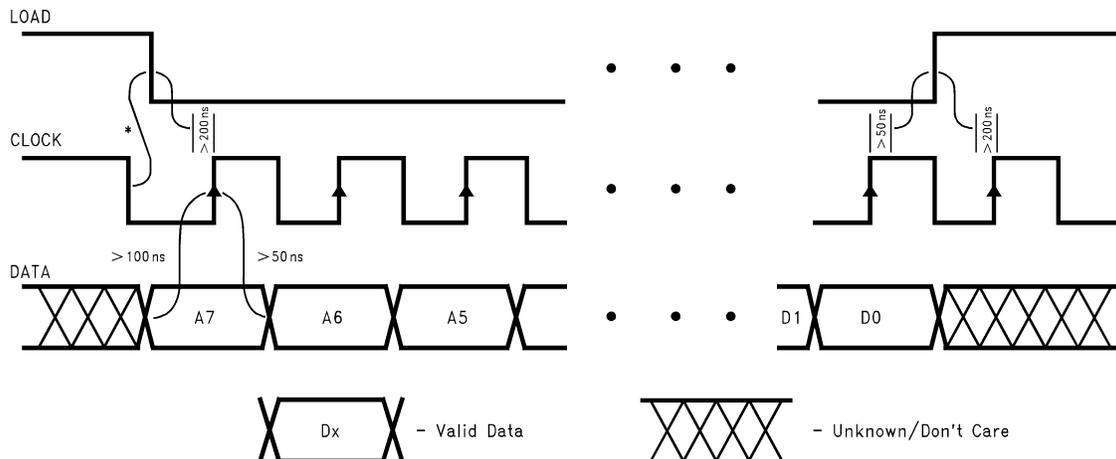
**\*Note:** Load and clock falling edges can be coincident, however, the clock falling edge cannot be delayed more than 20 ns from the falling edge of load. It is preferable that the falling edge of clock occurs before the falling edge of load.
