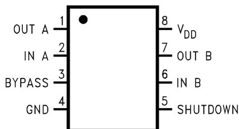
**Figure 1. Small Outline and PDIP Packages- Top View**
