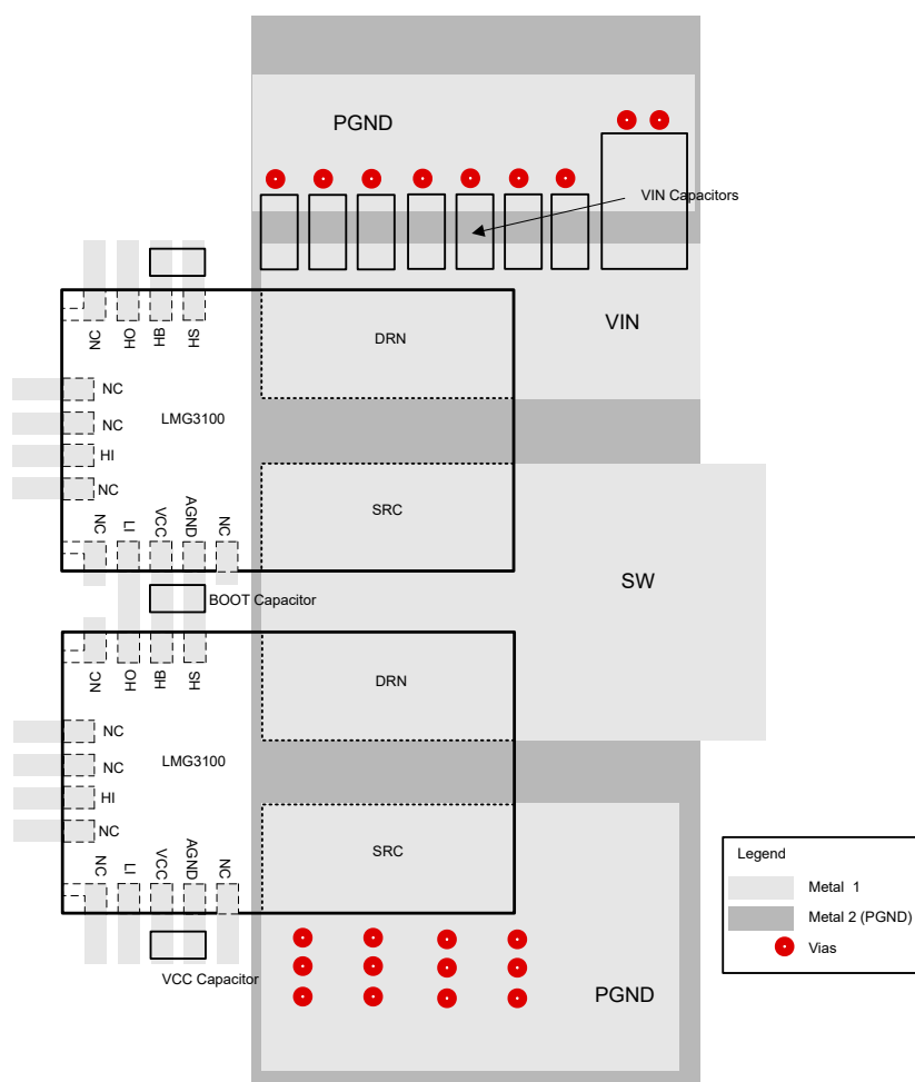
Figure 8-6. External Component Placement (Multi Layer Board)
