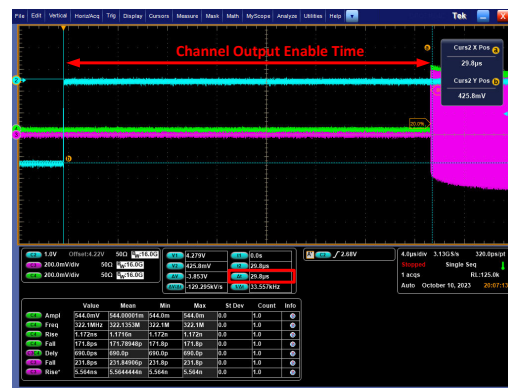
Figure 5-19. Channel Enable Setting Time
