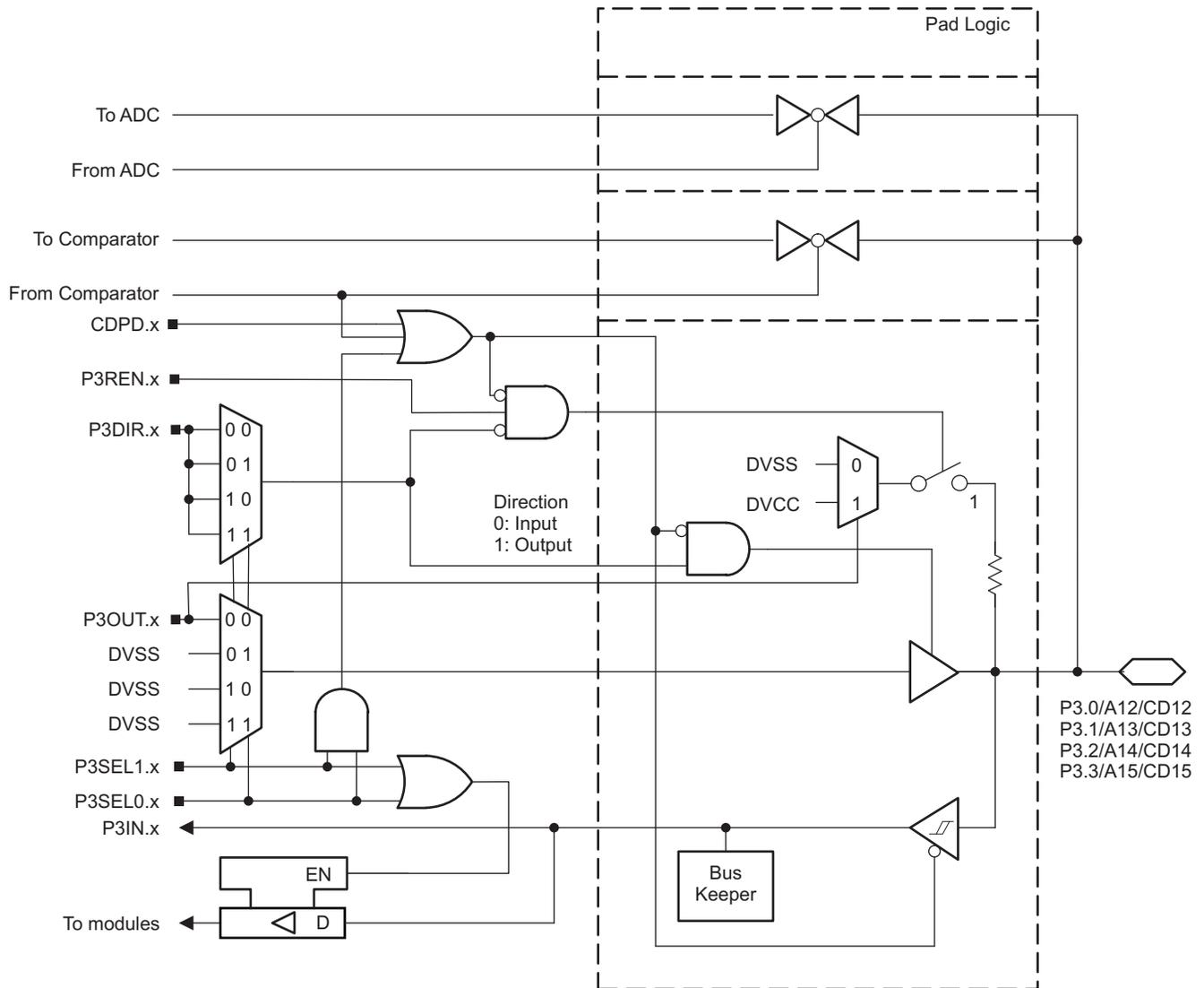
Figure 6-16. Port P3 (P3.0 to P3.3) Diagram
