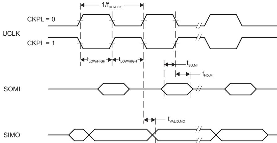
**Figure 5-6. SPI Master Mode, CKPH = 0**
