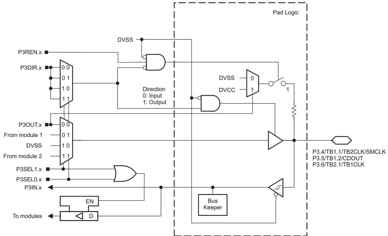
Figure 6-17. Port P3 (P3.4 to P3.6) Diagram
