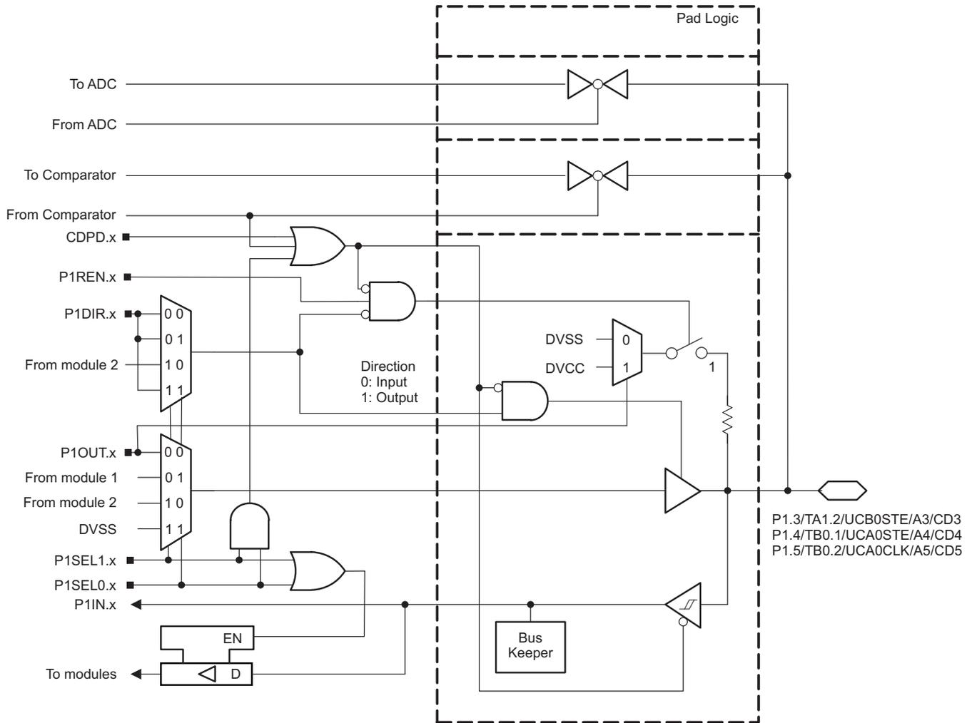
Figure 6-10. Port P1 (P1.3 to P1.5) Diagram
