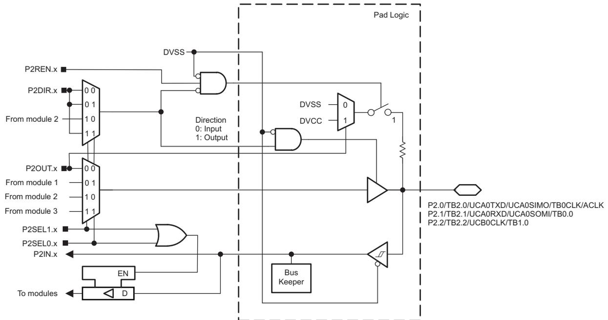
Figure 6-12. Port P2 (P2.0 to P2.2) Diagram
