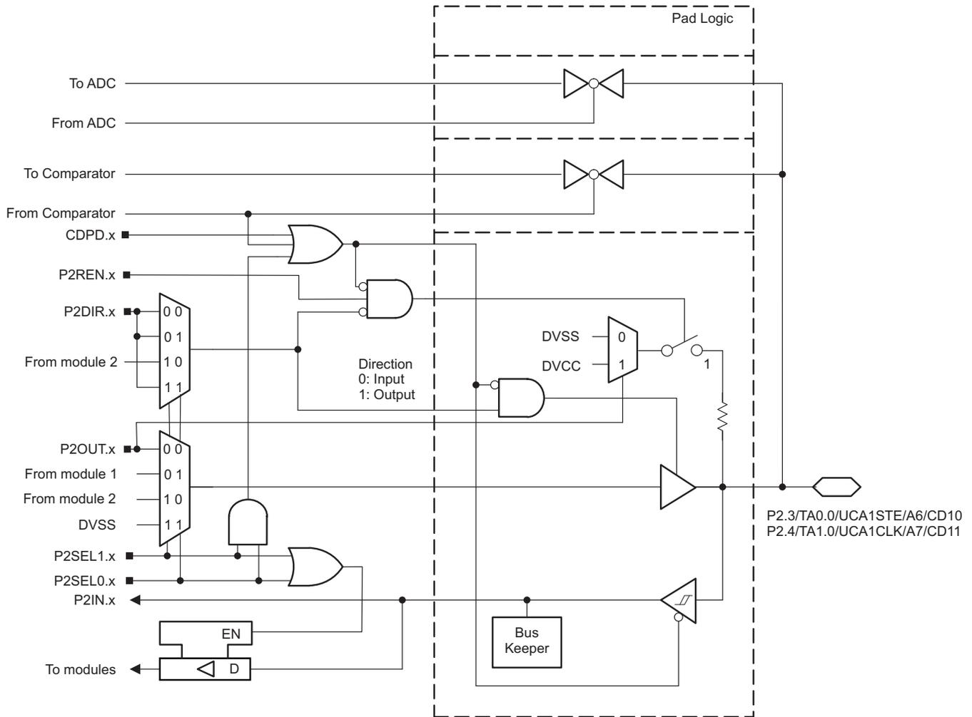
Figure 6-13. Port P2 (P2.3 and P2.4) Diagram
