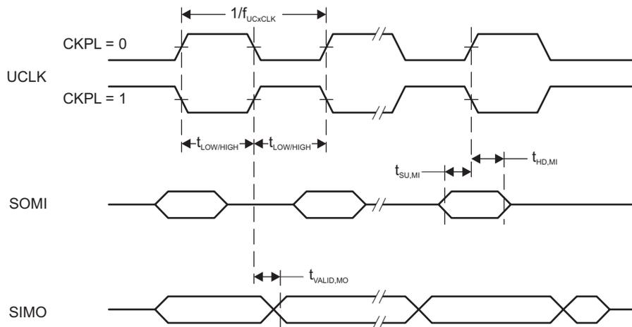
**Figure 5-7. SPI Master Mode, CKPH = 1**
