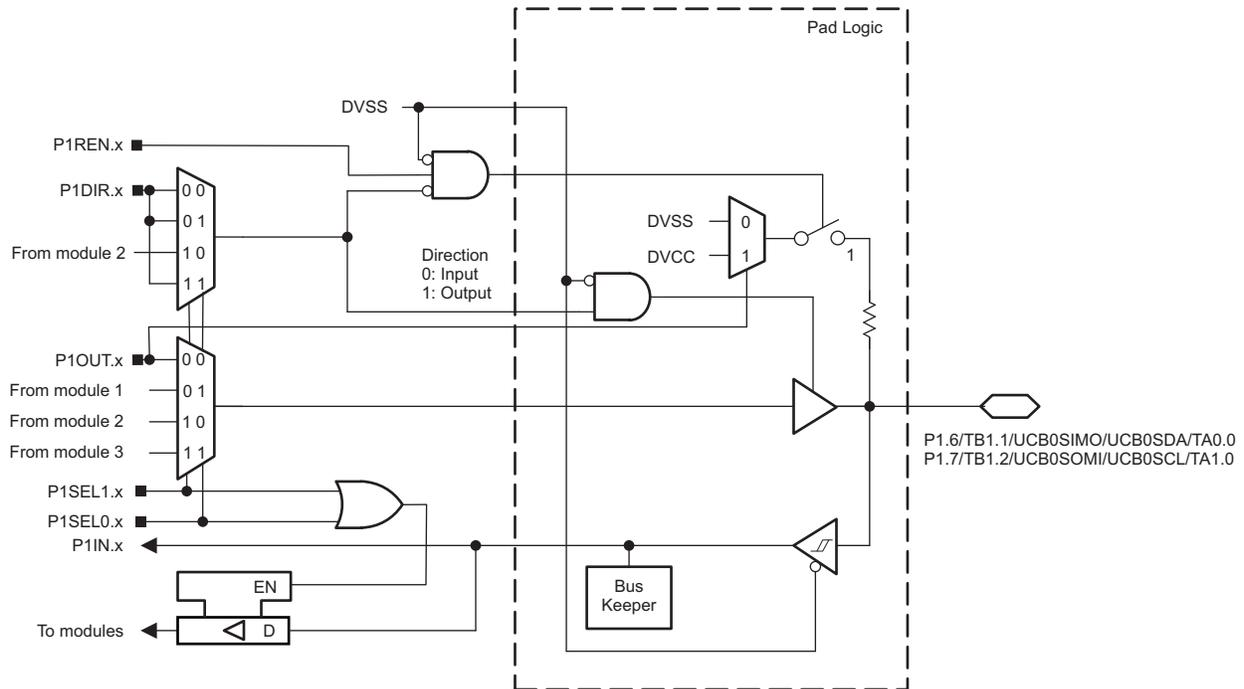
Figure 6-11. Port P1 (P1.6 and P1.7) Diagram
