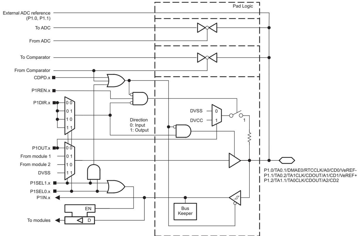
Figure 6-9. Port P1 (P1.0 to P1.2) Diagram
