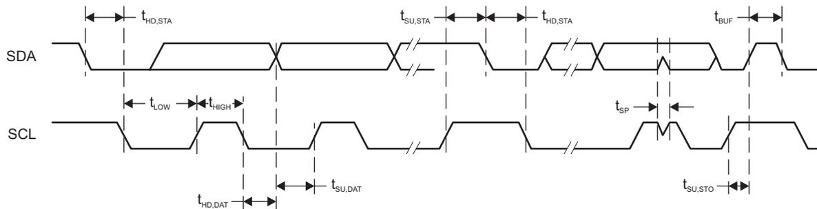
Figure 5-10. I<sup>2</sup>C Mode Timing
