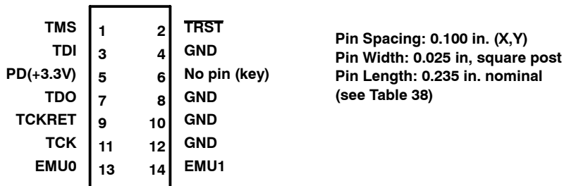
Figure 124. Target System Header
