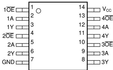
**Figure 5-1. D, DB, N, NS, PW, or J Package
