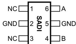
Figure 6-1. DBV Package, 6-Pin SOT-23 (Top View)
