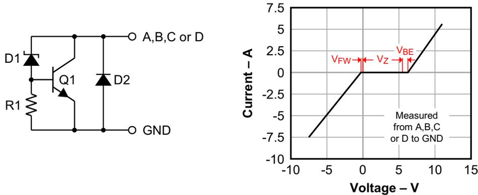
Figure 9-1. TVS Structure and Current — Voltage Characteristic
