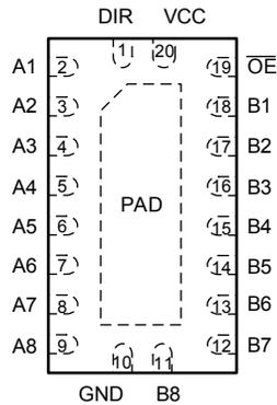
Figure 5-1. RKS Package, 20-Pin VQFN (Top View)
