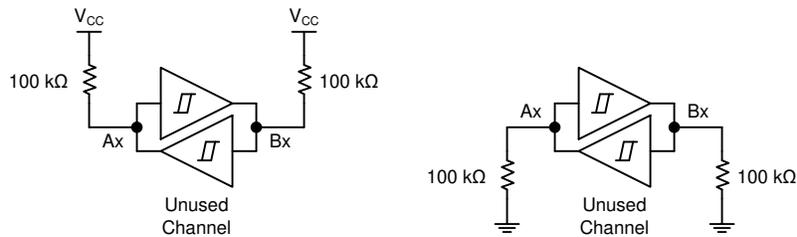
**Figure 8-2. Proper termination of unused transceiver channels**
