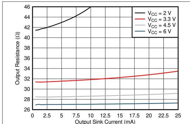
Figure 6-1. Output Driver Resistance in LOW State
