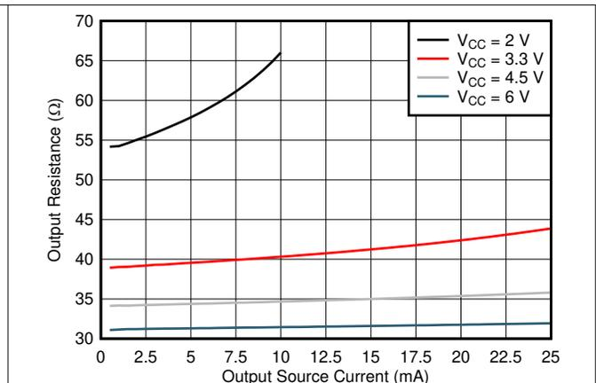
Figure 6-2. Output Driver Resistance in HIGH State.
