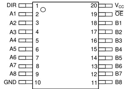
Figure 5-2. DGS Package, 20-Pin SOT (Top View)
