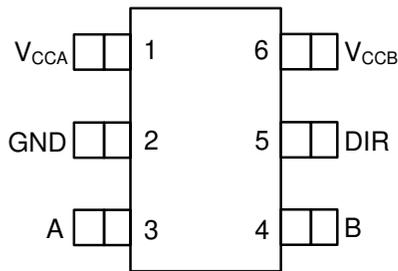
Figure 5-1. DBV 6-Pin SOT-23
