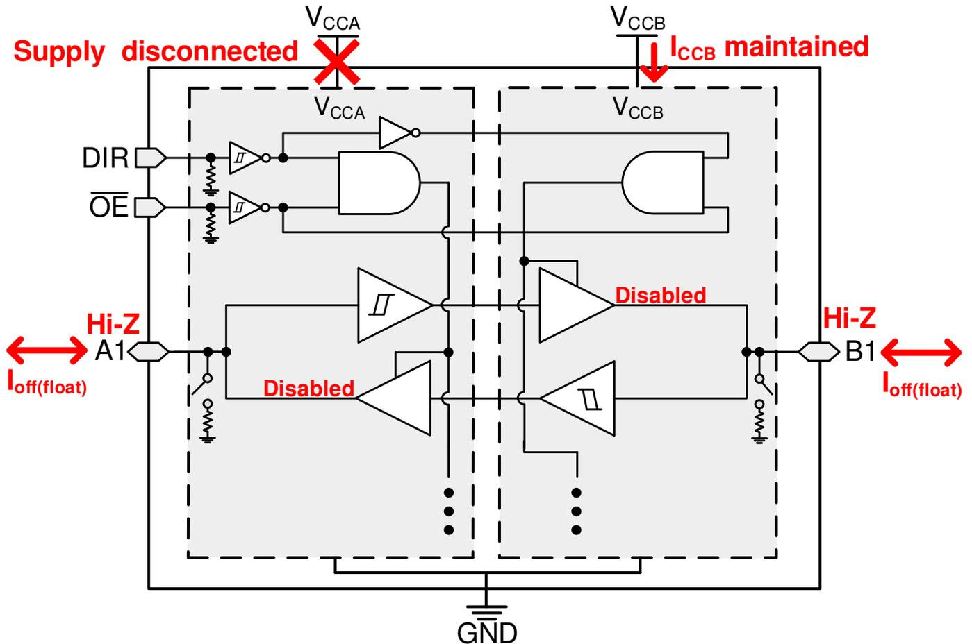
Figure 8-1. V<sub>CC</sub> Disconnect Feature
