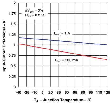
Figure 6-3. Dropout Voltage
