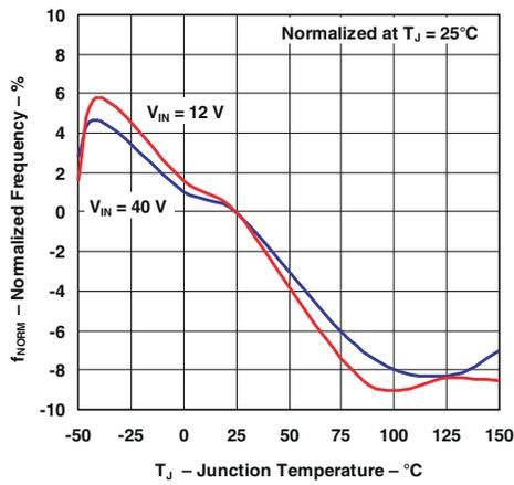
**Figure 6-7. Oscillator Frequency**
