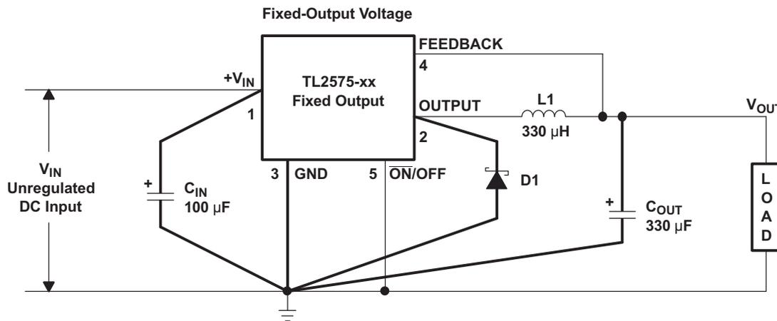
$C_{IN} = 100 \mu\text{F}$ , Aluminum Electrolytic
