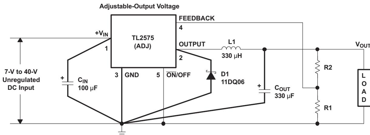
$$V_{OUT} = V_{REF} (1 + R2 / R1) = 5 \text{ V}$$
