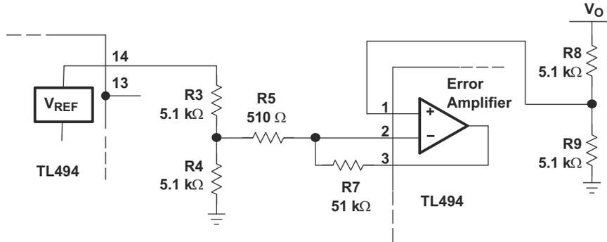
**Figure 10-3. Error-Amplifier Section**
