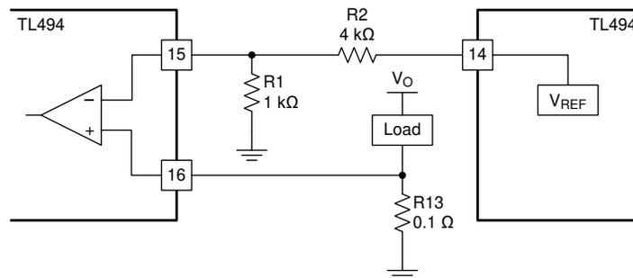
**Figure 10-4. Current-Limiting Circuit**
