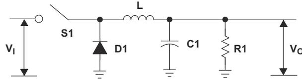
Figure 10-6. Switching Circuit
