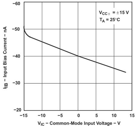
Figure 5-6. TLE2024xM Input Bias Current vs Common-Mode Input Voltage
