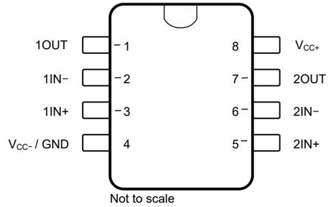
**Figure 4-2. TLE2022xM: JG Package, 8-Pin CDIP (Top View)**
