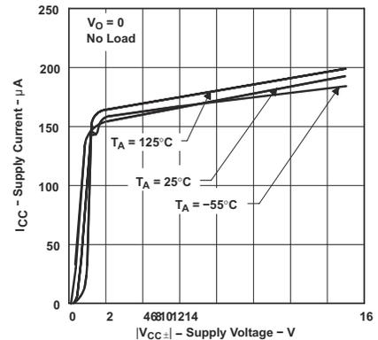
**Figure 5-34. TLE2021xM Supply Current vs Supply Voltage**
