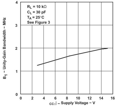
**Figure 5-57. TLE2021xM Unity-Gain Bandwidth vs Supply Voltage**
