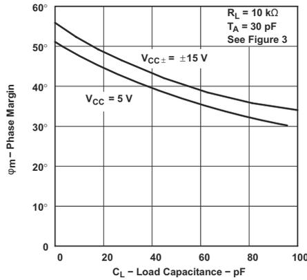
Figure 5-63. TLE2021xM Phase Margin vs Load Capacitance
