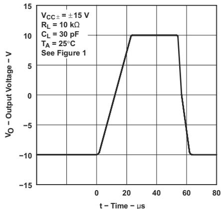
Figure 5-53. TLE2024xM Voltage-Follower Large-Signal Pulse Response
