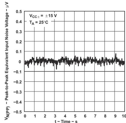
Figure 5-54. Peak-to-Peak Equivalent Input Noise Voltage 0.1Hz to 1Hz
