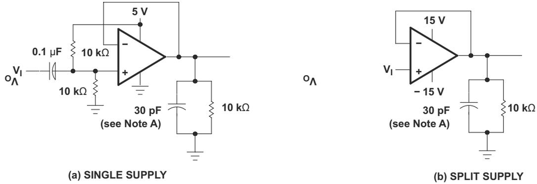
A.  $C_L$  includes fixture capacitance.
