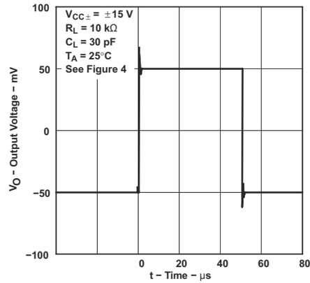
**Figure 5-46. Voltage-Follower Small-Signal Pulse Response**
