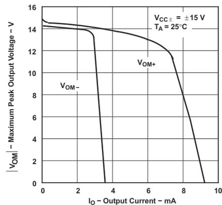
**Figure 5-11. TLE2021xM Maximum Peak Output Voltage vs Output Current**
