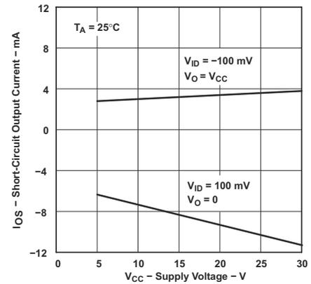
**Figure 5-28. TLE2021xM Short-Circuit Output Current vs Supply Voltage**
