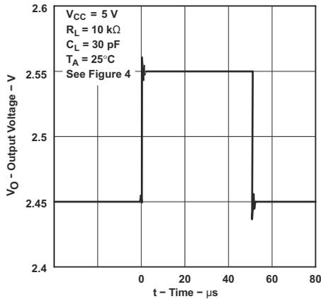
**Figure 5-47. Voltage-Follower Small-Signal Pulse Response**
