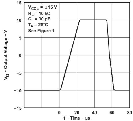
Figure 5-52. TLE2022xM Voltage-Follower Large-Signal Pulse Response
