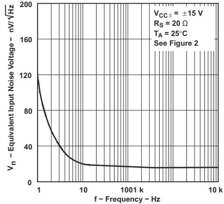
**Figure 5-56. Equivalent Input Noise Voltage vs Frequency**
