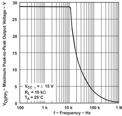
**Figure 5-21. Maximum Peak-to-Peak Output Voltage vs Frequency**
