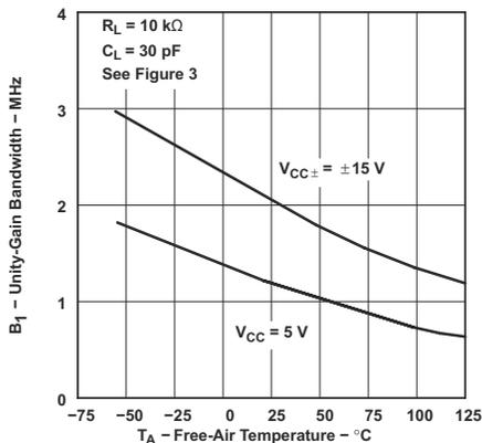
Data at high and low temperatures applicable only within rated operating free-air temperature ranges of the various devices
