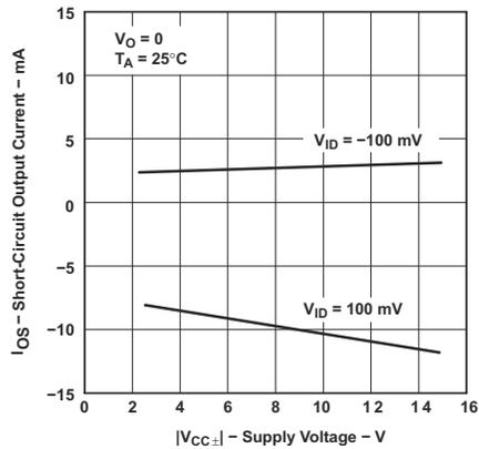
**Figure 5-27. TLE2022xM and TLE2024xM Short-Circuit Output Current vs Supply Voltage**
