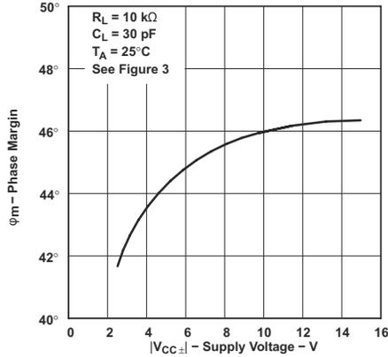
Figure 5-61. TLE2021xM Phase Margin vs Supply Voltage
