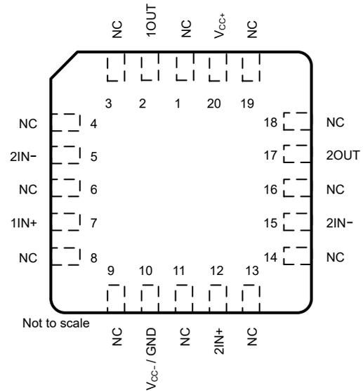
**Figure 4-4. TLE2022xM: FK Package, 20-Pin LCCC (Top View)**
