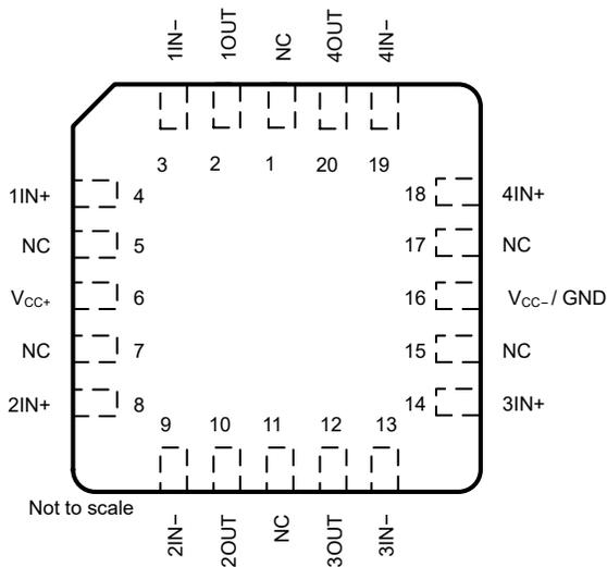
**Figure 4-5. TLE2024xM: FK Package, 20-Pin LCCC (Top View)**
