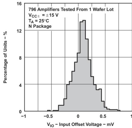
Figure 5-3. Distribution of TLE2024xM Input Offset Voltage
