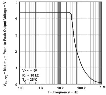
**Figure 5-20. Maximum Peak-to-Peak Output Voltage Vs Frequency**
