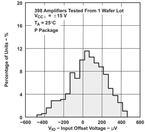
Figure 5-2. Distribution of TLE2022xM Input Offset Voltage
