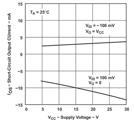
**Figure 5-29. TLE2022xM and TLE2024xM Short-Circuit Output Current vs Supply Voltage**
