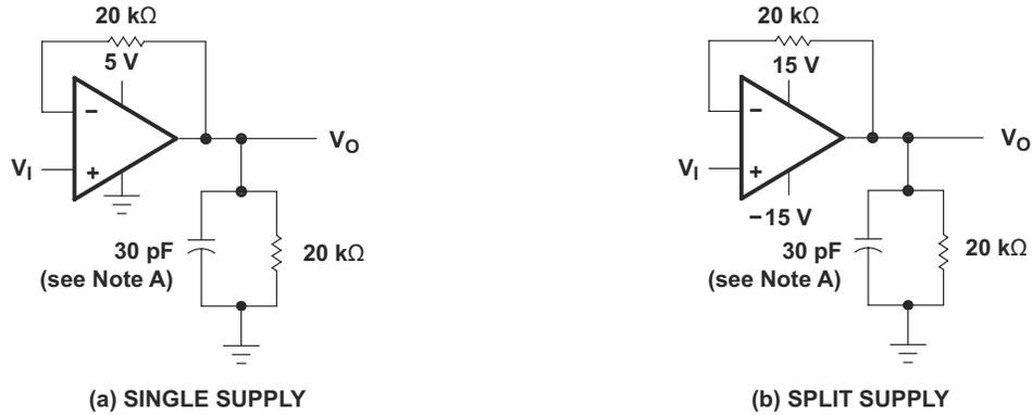
A.  $C_L$  includes fixture capacitance.
