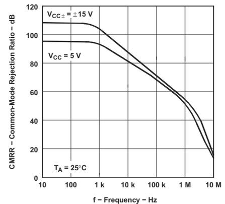
**Figure 5-42. TLE2024xM Common-Mode Rejection Ratio vs Frequency**
