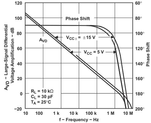
**Figure 5-22. Large-Signal Differential Voltage Amplification and Phase Shift vs Frequency**
