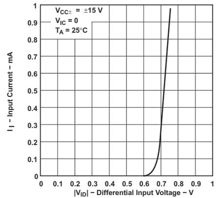
**Figure 5-10. Input Current vs Differential Input Voltage**
