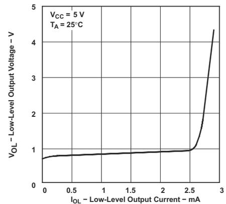
**Figure 5-18. Low-Level Output Voltage vs Low-Level Output Current**
