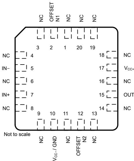
**Figure 4-3. TLE2021xM: FK Package, 20-Pin LCCC (Top View)**
