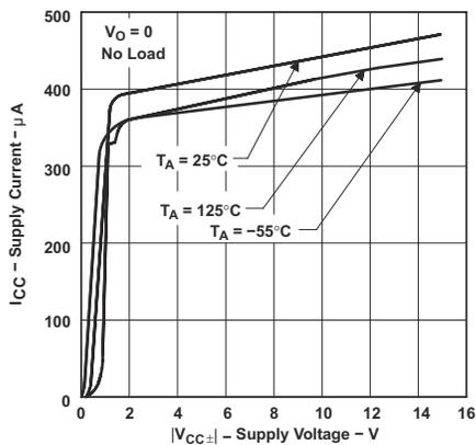
**Figure 5-35. TLE2022xM Supply Current vs Supply Voltage**
