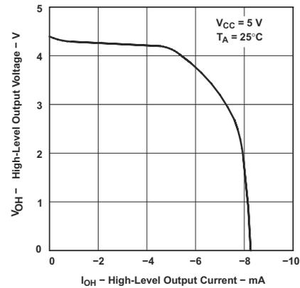
**Figure 5-16. TLE2022xM and TLE2024xM High-Level Output Voltage vs High-Level Output Current**
