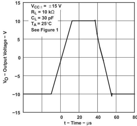
Figure 5-51. TLE2021xM Voltage-Follower Large-Signal Pulse Response
