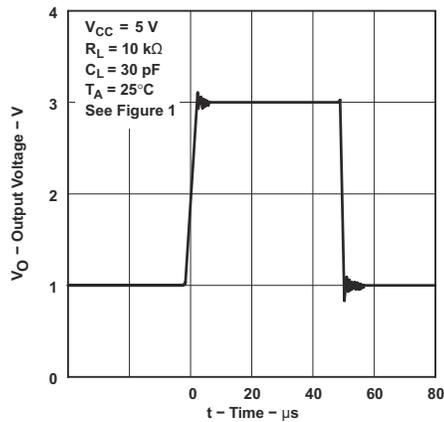
**Figure 5-48. TLE2021xM Voltage-Follower Large-Signal Pulse Response**
