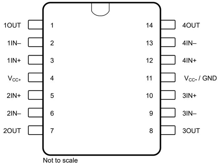
**Figure 4-6. TLE2024xM: J Package, 14-Pin CDIP (Top View)**
