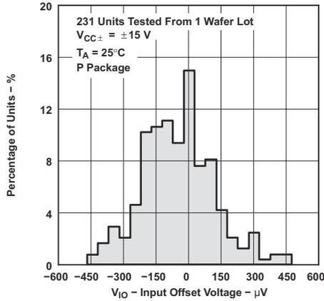
Figure 5-1. Distribution of TLE2021xM Input Offset Voltage
