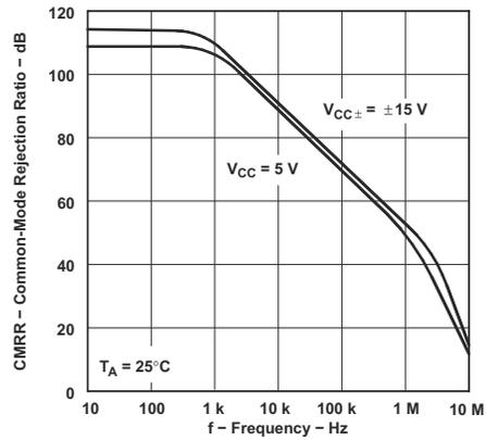
**Figure 5-40. TLE2021xM Common-Mode Rejection Ratio vs Frequency**
