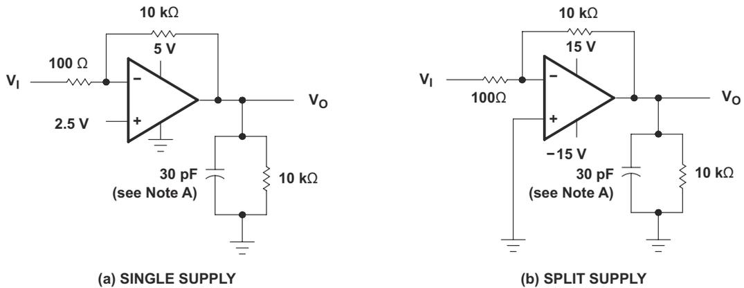
A.  $C_L$  includes fixture capacitance.
