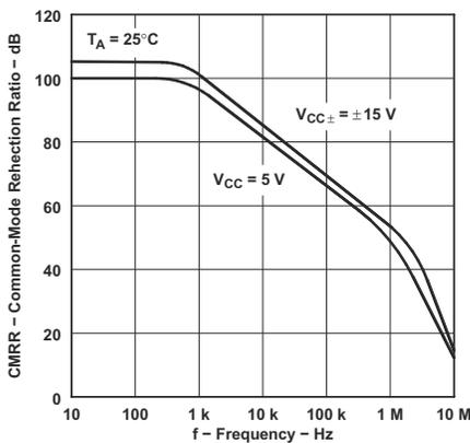
**Figure 5-41. TLE2022xM Common-Mode Rejection Ratio vs Frequency**
