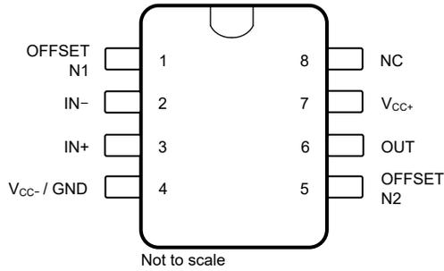
**Figure 4-1. TLE2021xM: JG Package, 8-Pin CDIP (Top View)**
