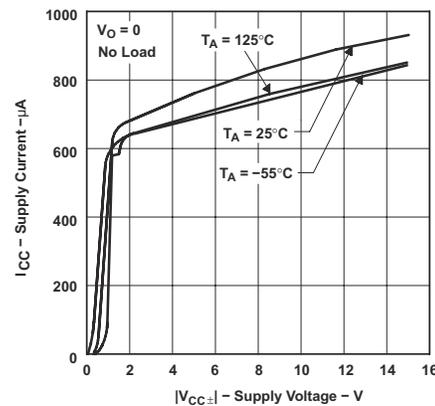
**Figure 5-36. TLE2024xM Supply Current vs Supply Voltage**
