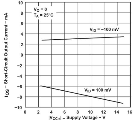
**Figure 5-26. TLE2021xM Short-Circuit Output Current vs Supply Voltage**
