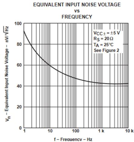
Figure 5-12. Equivalent Input Noise Voltage vs Frequency
