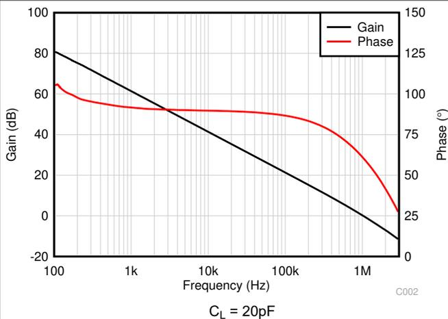
Figure 5-17. Open-Loop Gain and Phase vs Frequency
