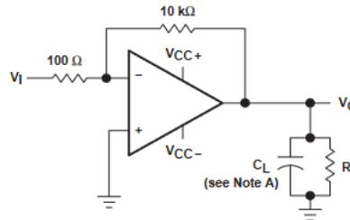
Figure 6-3. Unity-Gain Bandwidth and Phase-Margin Test Circuit
