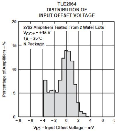
Figure 5-3. TLE2064 Distribution of Input Offset Voltage
