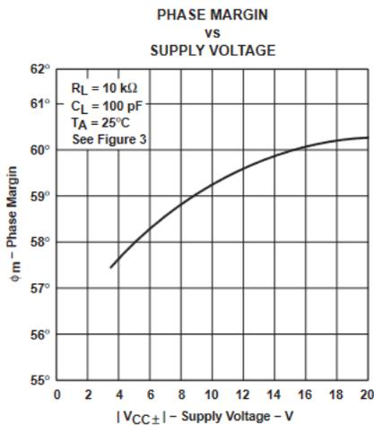
Figure 5-15. Phase Margin vs Supply Voltage
