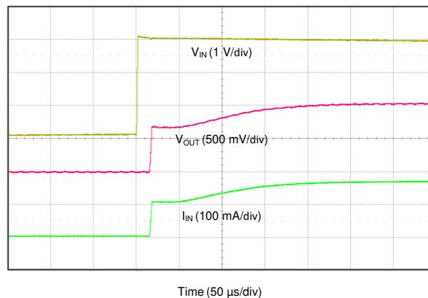
**Figure 8-5. No Inrush Startup, 3.0-V to 1.0-V Regulation**
