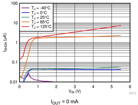
**Figure 6-4. Shutdown Current vs  $V_{IN}$  and Temperature**
