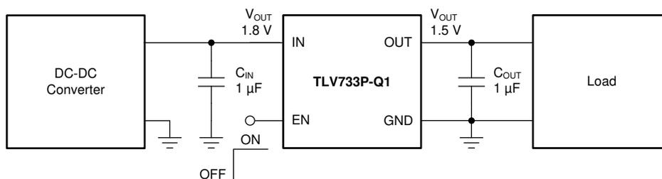
Figure 8-2. DC-DC Converter Post Regulation
