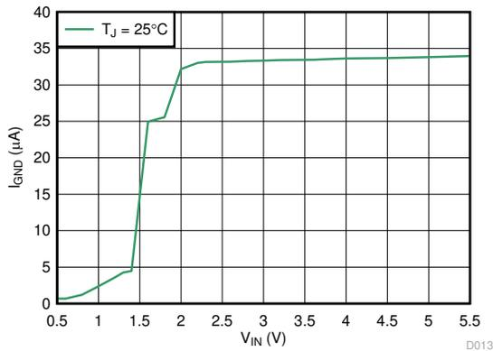
**Figure 6-3. Ground Pin Current vs  $V_{IN}$**
