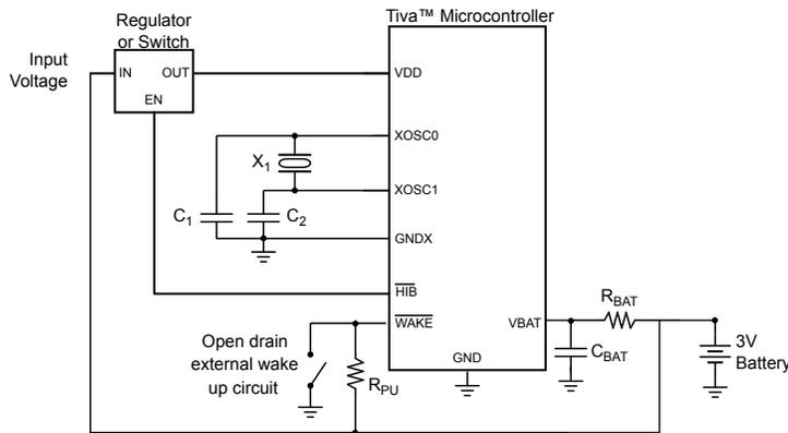
**Note:** Some devices may not supply the GNDX signal. If GNDX is absent, the crystal load capacitors can be tied to GND externally. See “Signal Tables” on page 1076 for pins specific to your device.
