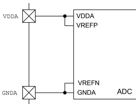
The range of this conversion value is from 0x000 to 0xFFFF. In single-ended-input mode, the 0x000 value corresponds to the voltage level on VREFN; the 0xFFFF value corresponds to the voltage level on VREFP. This configuration results in a resolution that can be calculated using the following equation:
