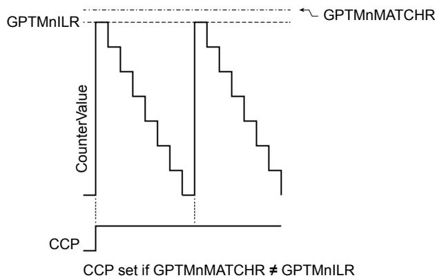
Figure 11-7 on page 683 shows how the CCP output operates when the  $PLO$  and  $MRSU$  bits are set and the **GPTMTnMATCHR** value is the same as the **GPTMTnILR** value. In this situation, if the  $PLO$  bit is 0, the CCP signal goes high when the **GPTMTnILR** value is loaded and the match would be essentially ignored.
