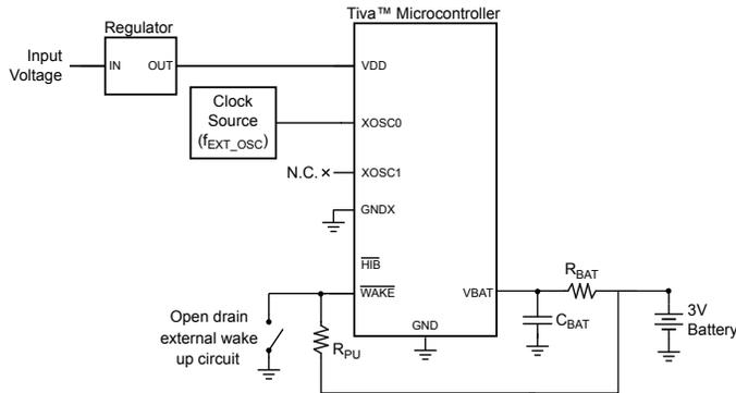
**Note:** Some devices may not supply the GNDX,  $\overline{\text{WAKE}}$  or  $\overline{\text{HIB}}$  signals. See “Signal Tables” on page 1076 for pins specific to your device.
