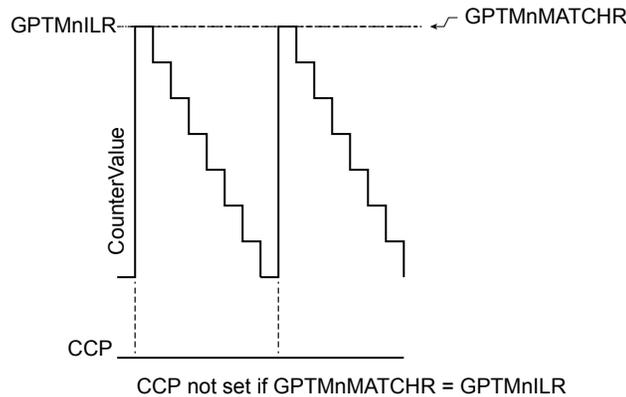
Figure 11-8 on page 683 shows how the CCP output operates when the `PLO` and `MRSU` bits are set and the `GPTMTnILR` is greater than the `GPTMTnMATCHR` value.
