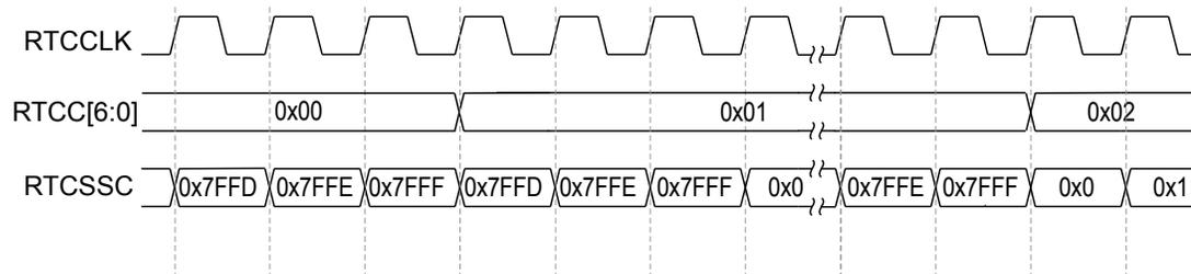
In the case of a trim value below `0x7FFF`, the `RTCSSC` value is advanced from `0x7FFF` to the trim value while the `RTCC` value is incremented from `0x0` to `0x1`. If the match value is within that range, the match interrupt is not triggered. For example, as shown in Figure 7-6 on page 465, if the match interrupt was configured with `RTCM0=0x1` and `RTCSSM=0x2`, an interrupt would never be triggered.
