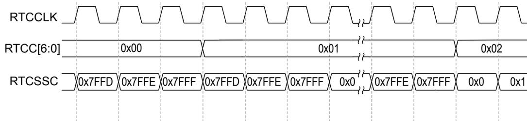
In the case of a trim value below `0x7FFF`, the `RTCSSC` value is advanced from `0x7FFF` to the trim value while the `RTCC` value is incremented from `0x0` to `0x1`. If the match value is within that range, the match interrupt is not triggered. For example, as shown in Figure 7-6 on page 483, if the match interrupt was configured with `RTCM0=0x1` and `RTCSSM=0x2`, an interrupt would never be triggered.
