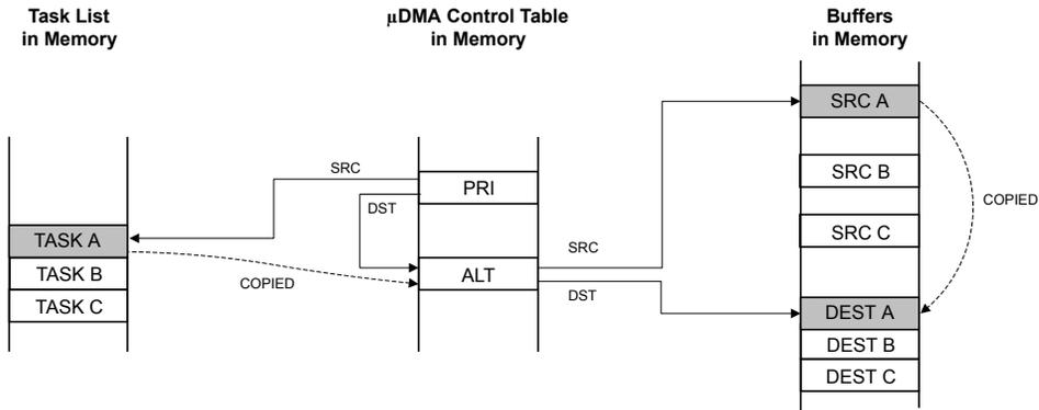
Using the channel's primary control structure, the  $\mu$ DMA controller copies task A configuration to the channel's alternate control structure.
