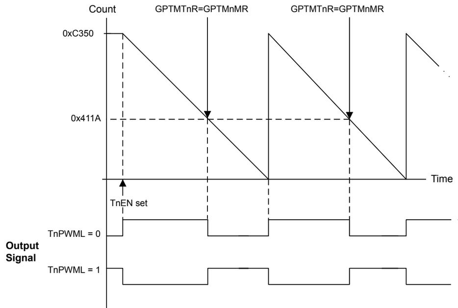
When synchronizing the timers using the **GPTMSYNC** register, the timer must be properly configured to avoid glitches on the CCP outputs. Both the  $TnPLO$  and the  $TnMRSU$  bits must be set in the **GPTMTnMR** register. Figure 11-6 on page 703 shows how the CCP output operates when the  $TnPLO$  and  $TnMRSU$  bits are set and the **GPTMTnMATCHR** value is greater than the **GPTMTnILR** value.
