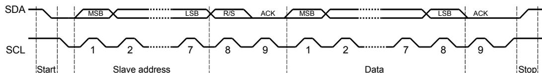
The first seven bits of the first byte make up the slave address (see Figure 16-5). The eighth bit determines the direction of the message. A zero in the R/S position of the first byte means that the
