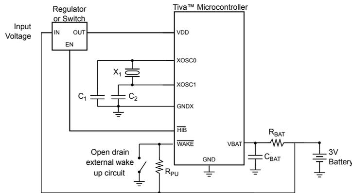
**Note:** Some devices may not supply the GNDX signal. If GNDX is absent, the crystal load capacitors can be tied to GND externally. See “Signal Tables” on page 1161 for pins specific to your device.
